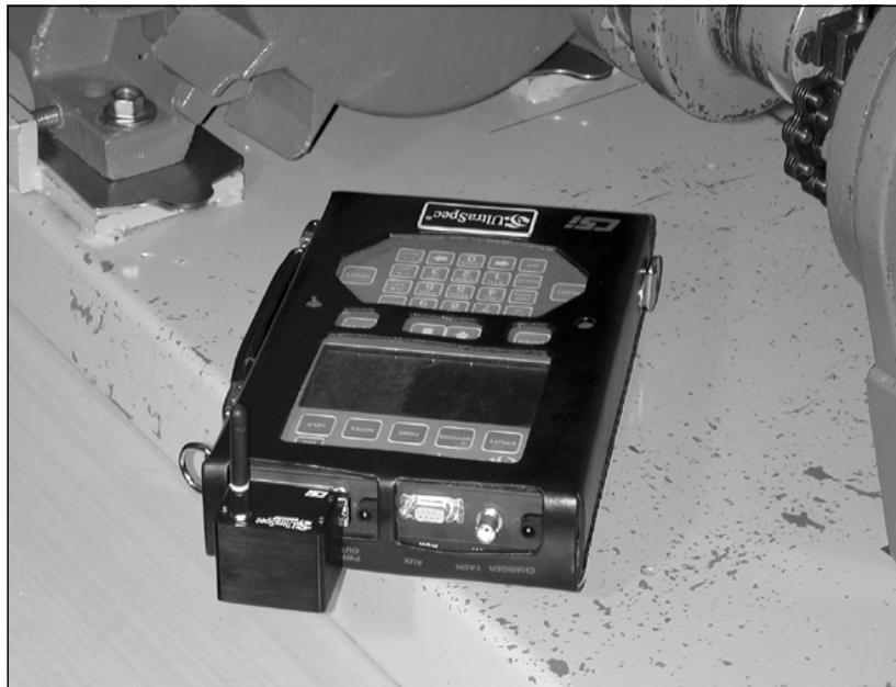
Attaching 8000RF to RS232 25-pin Serial Port
