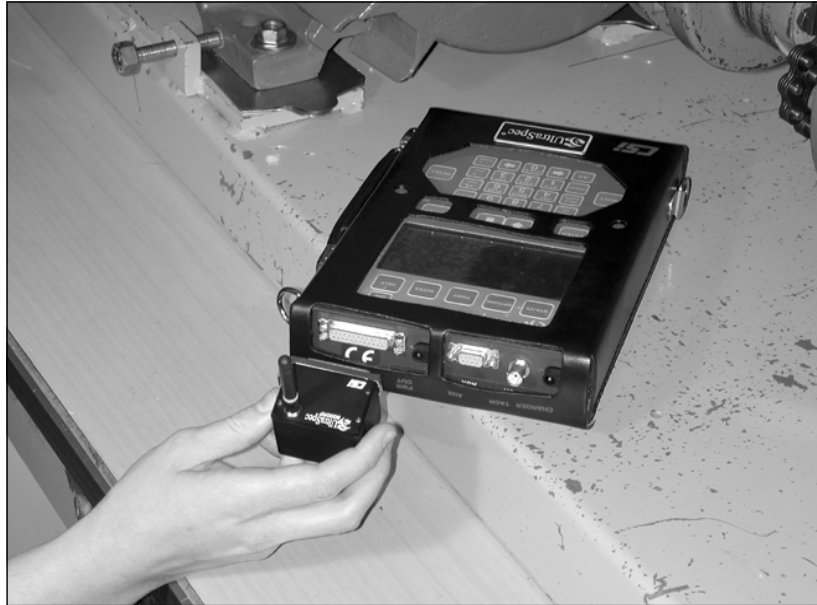
Attaching 8000RF to RS232 25-pin Serial Port
