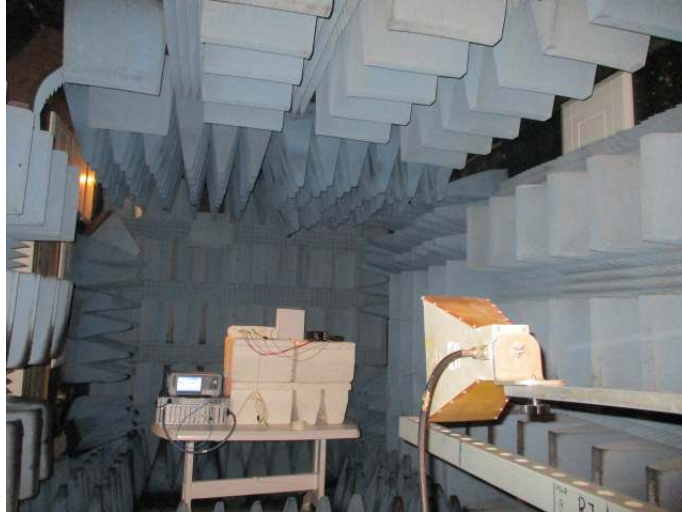
Figure 9. Radiated Emission Test 1.0 - 8.0GHz
