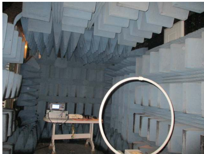
Figure 6. Radiated Emission Test 9kHz - 30MHz
