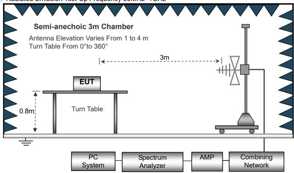
(C) Radiated Emission Test-Up Frequency Above 1GHz
