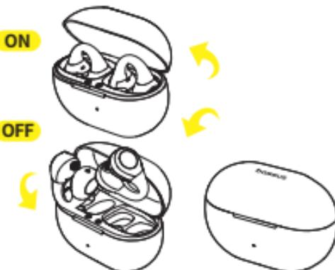
**Power on:** After the charging case is opened, the earbuds automatically enter the power-on state.
