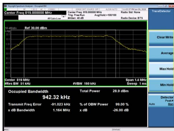
LTE Band 26 16QAM 1.4MHz CH Middle
