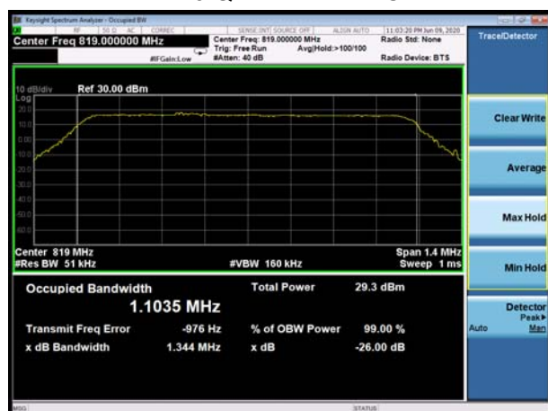
LTE Band 26 QPSK 5MHz CH Middle
