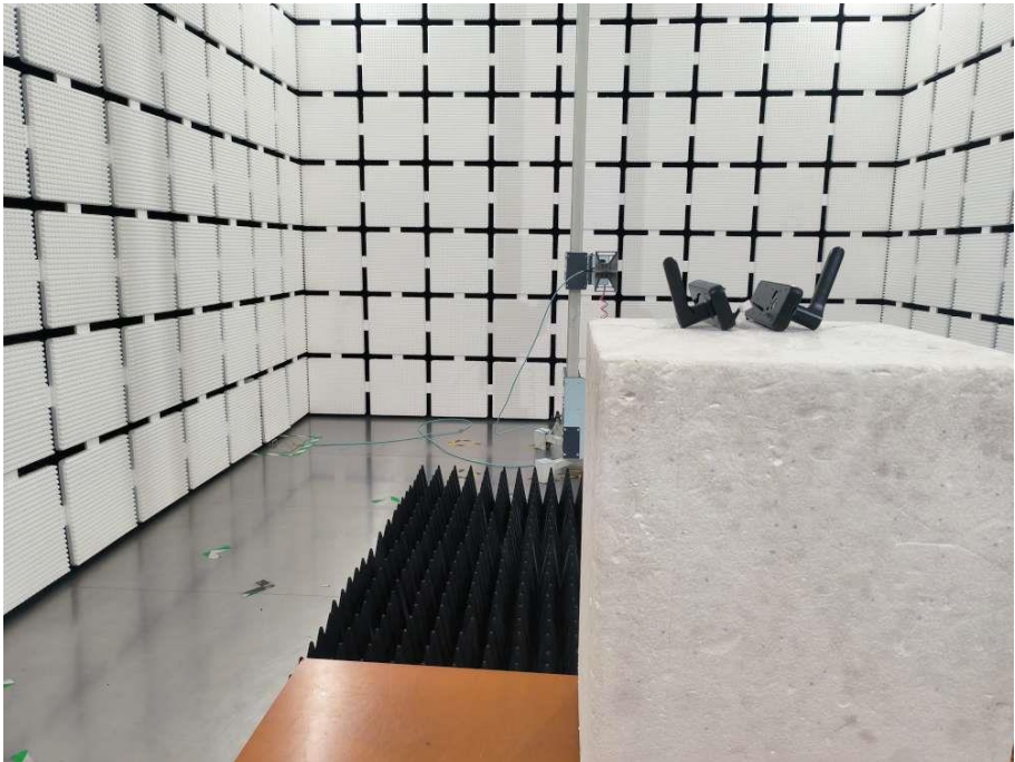
Radiated Emission Test View Above 1GHz
