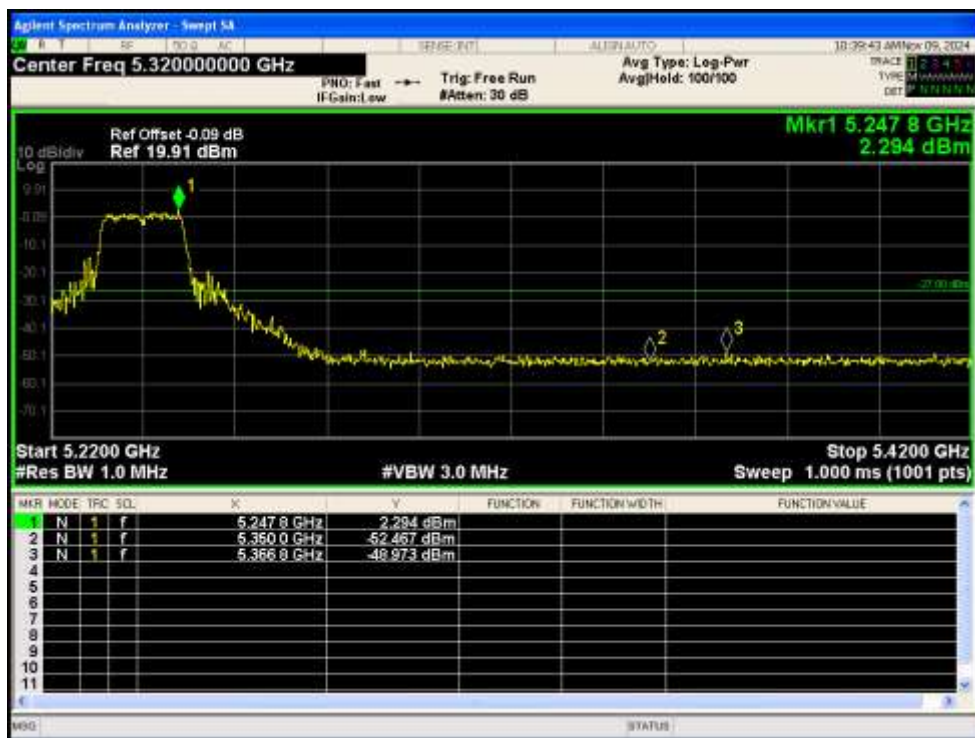
Band Edge NVNT n40 5190MHz Low Ant1
