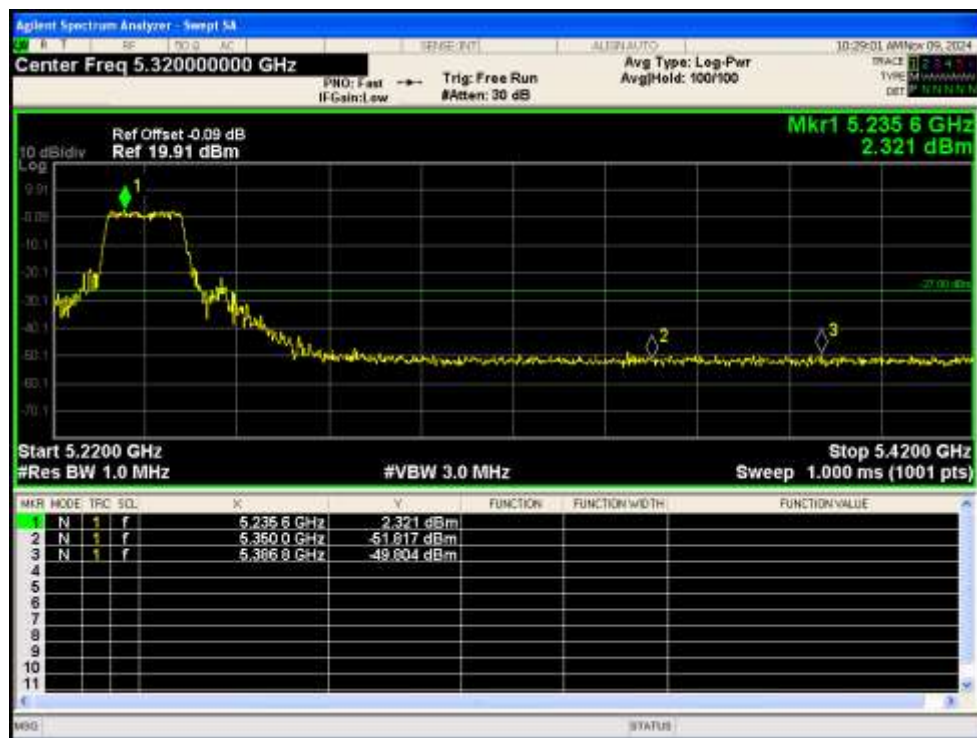
Band Edge NVNT ac20 5180MHz Low Ant1
