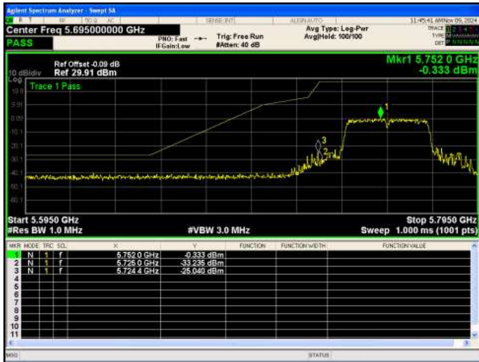
Band Edge NVNT n40 5795MHz High Ant1
