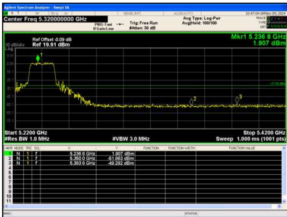
Band Edge NVNT ac40 5190MHz Low Ant1
