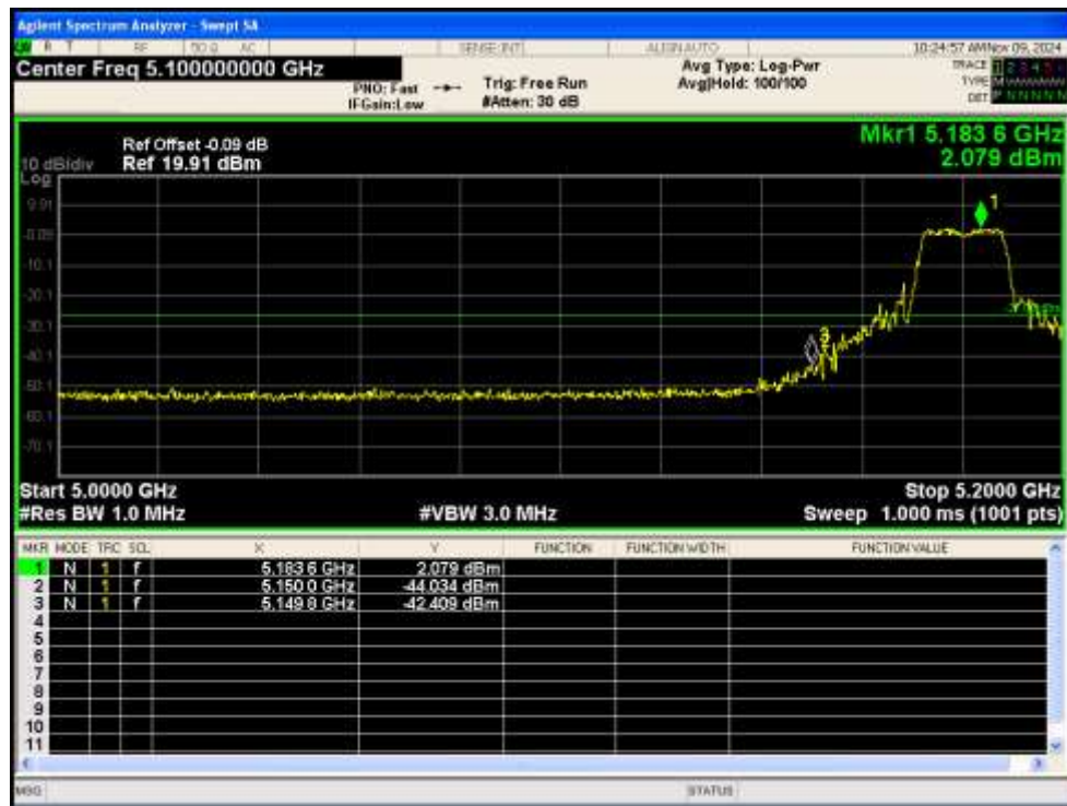
Band Edge NVNT a 5240MHz High Ant1
