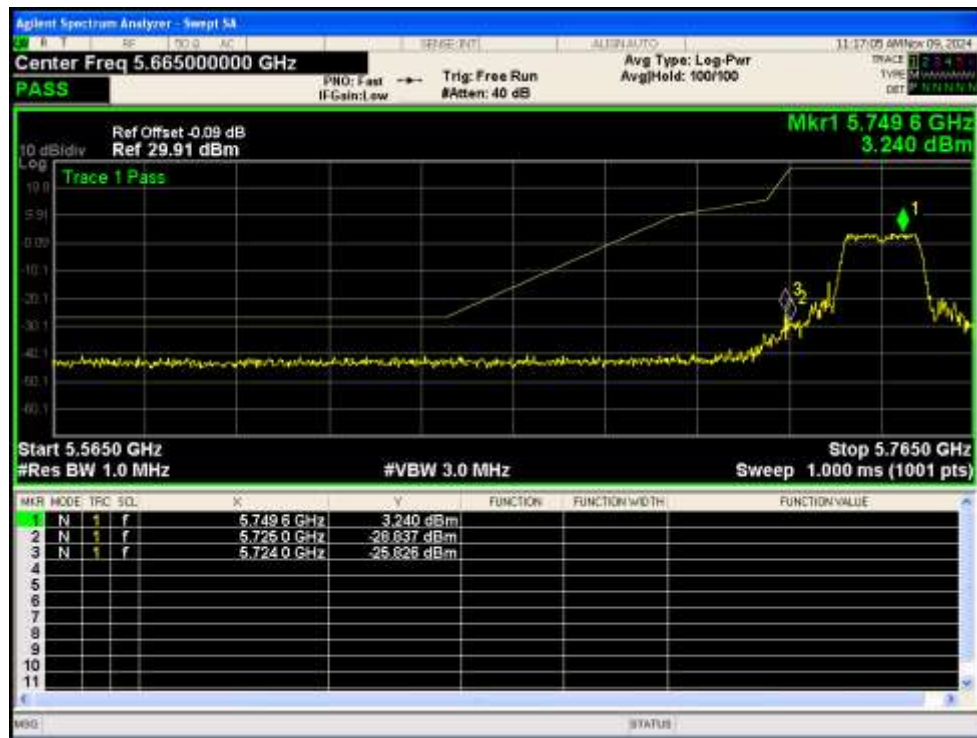
Band Edge NVNT a 5825MHz High Ant1
