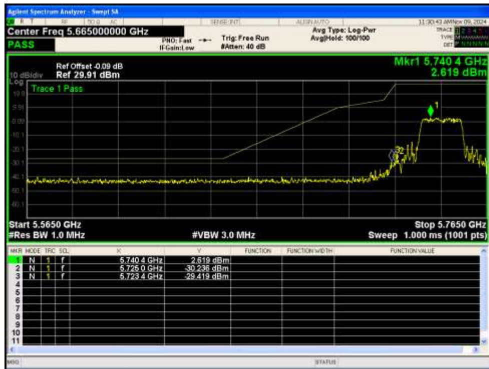
Band Edge NVNT n20 5825MHz High Ant1
