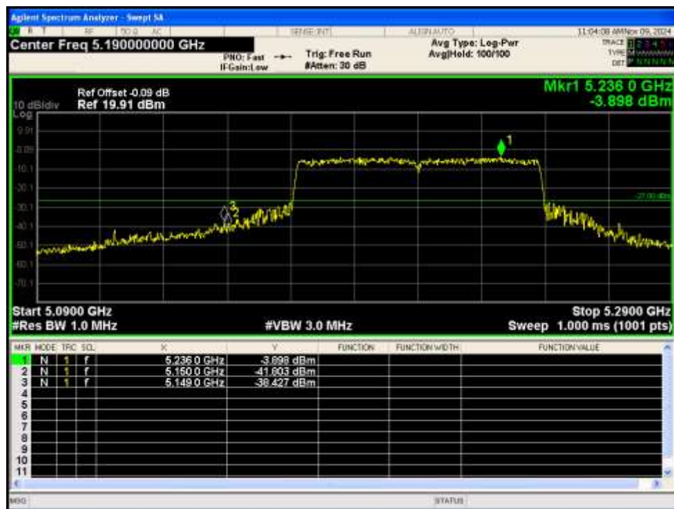
Band Edge NVNT n20 5180MHz Low Ant1
