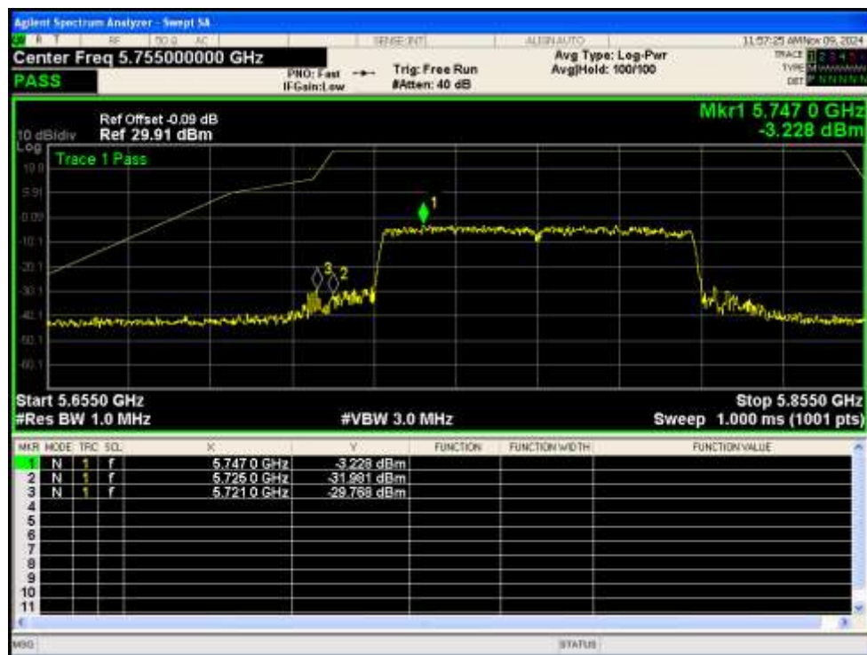
Band Edge NVNT n20 5745MHz Low Ant1
