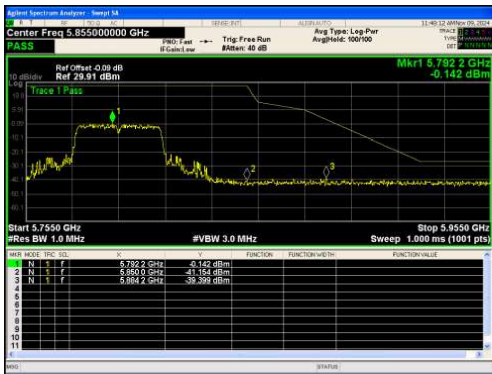
Band Edge NVNT n40 5795MHz High Ant1
