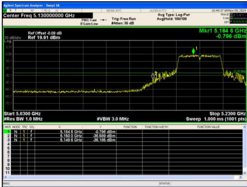
Band Edge NVNT n40 5230MHz High Ant1
