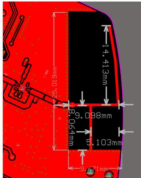
Antenna Module Peak Gain: ~1.5dBi (2 planes tested)
