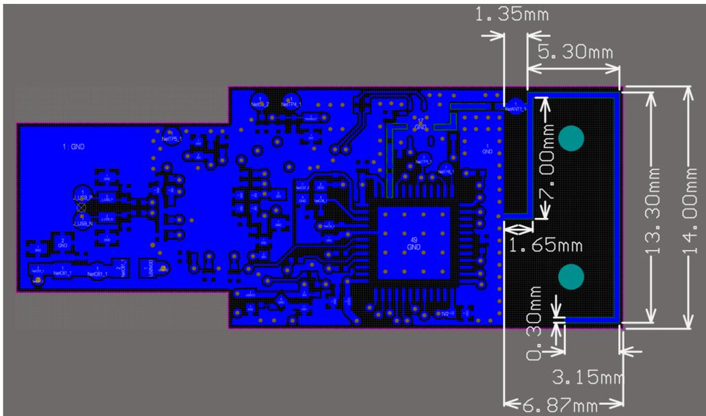
Antenna Module Peak Gain: ~5.8dBi (3 planes tested)
