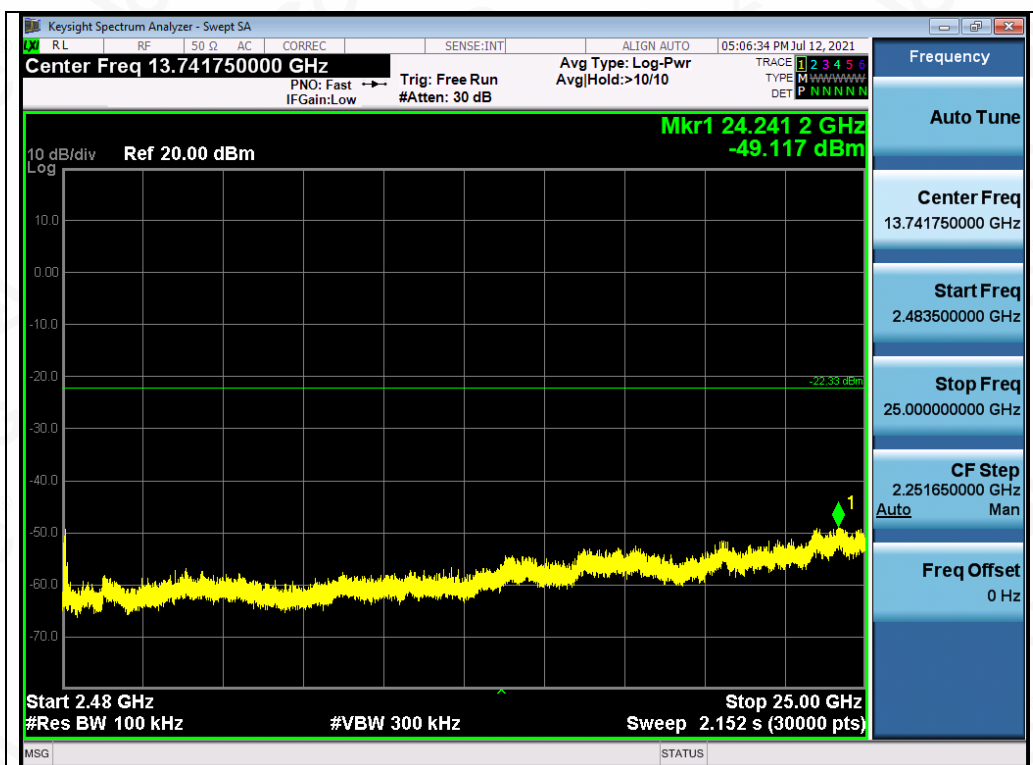
Test_Graph_BR_ANT1_2402_1Mbps_Higher Band Emissions
