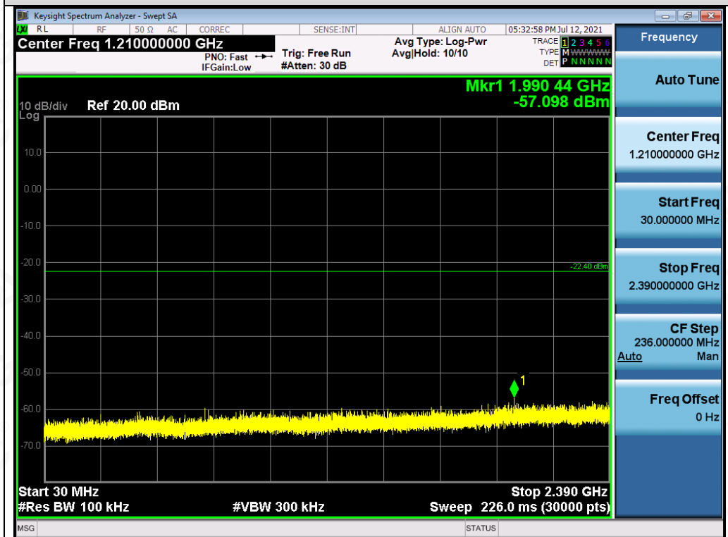
Test_Graph_EDR_ANT1_2402_3Mbps_Lower Band Emissions
