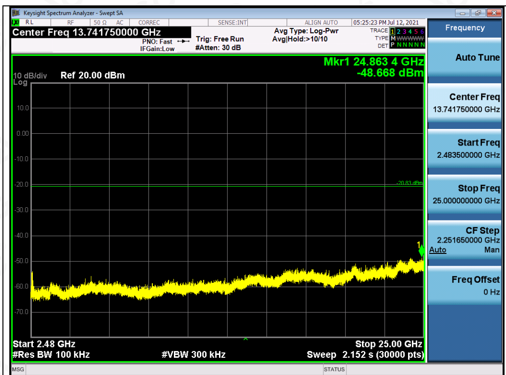
Test_Graph_EDR_ANT1_2441_2Mbps_Higher Band Emissions
