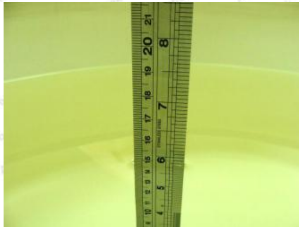
Photo of Liquid Height for Body SAR
