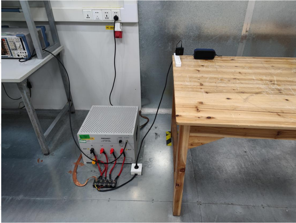
Photo of Conducted Emission Measurement
