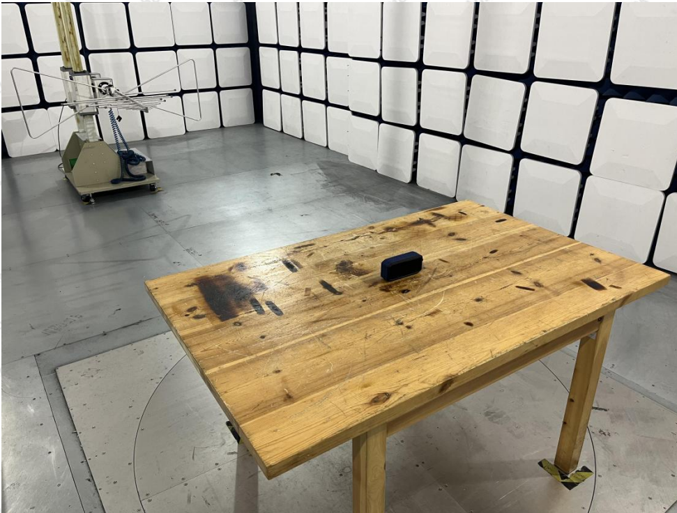
Photo of Radiation Emission Test
