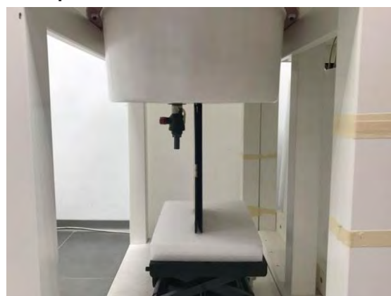
Fig.7 EUT Left side to flat phantom
