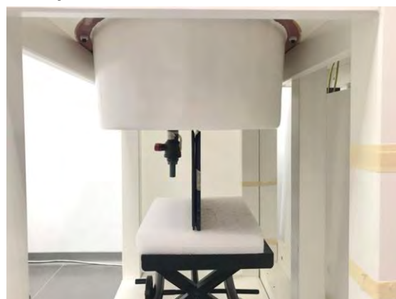
Fig.4 EUT Top side to flat phantom
