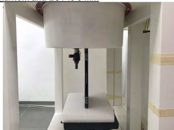
Fig.6 EUT Right side to flat phantom
