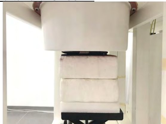
Fig.3 EUT Back side to flat phantom
