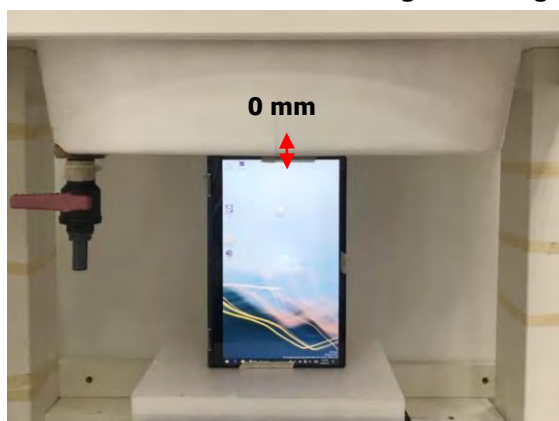
Fig.7 EUT Left side to flat phantom
