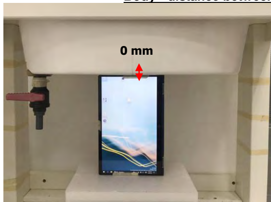
Fig.6 EUT Right side to flat phantom
