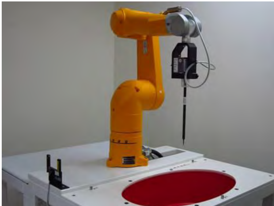
Fig.1 Photograph of the SAR measurement system
