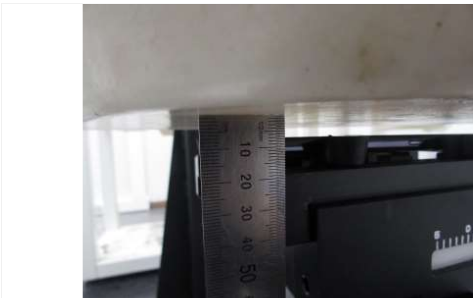
Distance of 7 mm from the EUT
