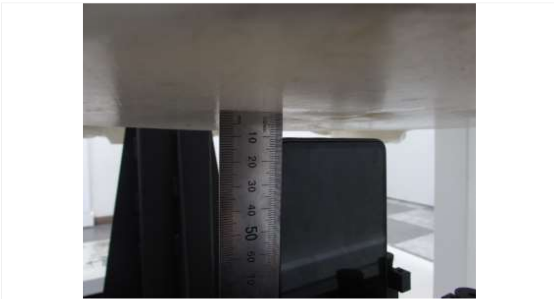
Distance of 10 mm from the EUT
