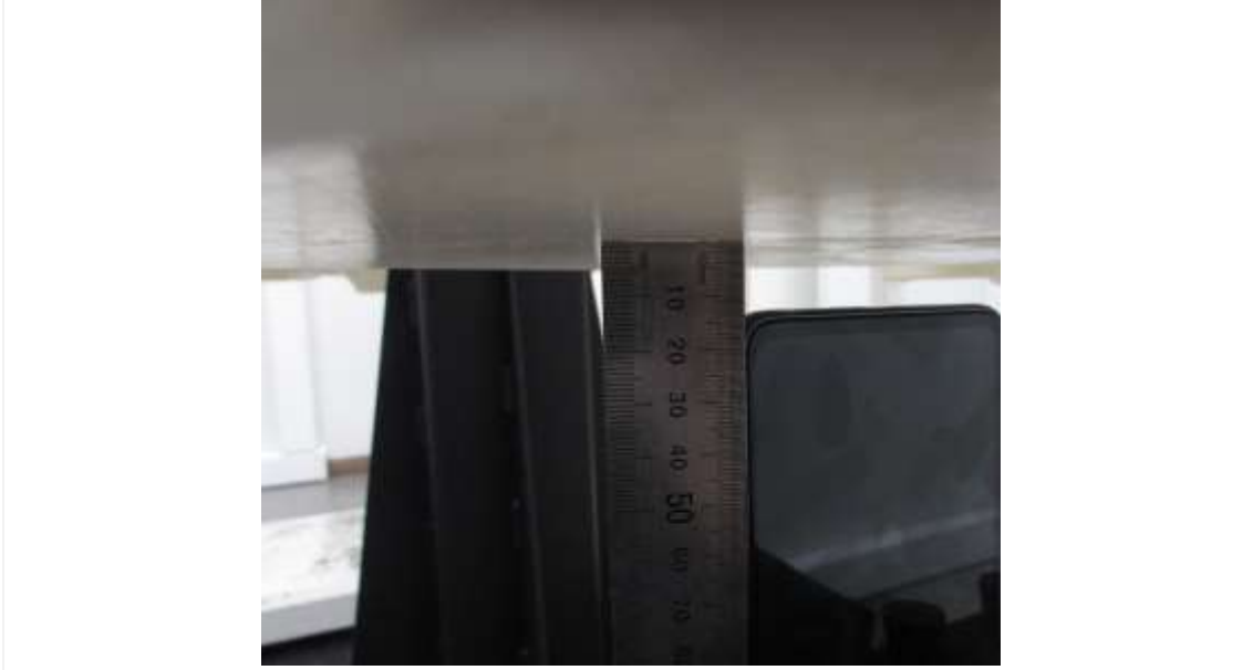
Distance of 13 mm from the EUT
