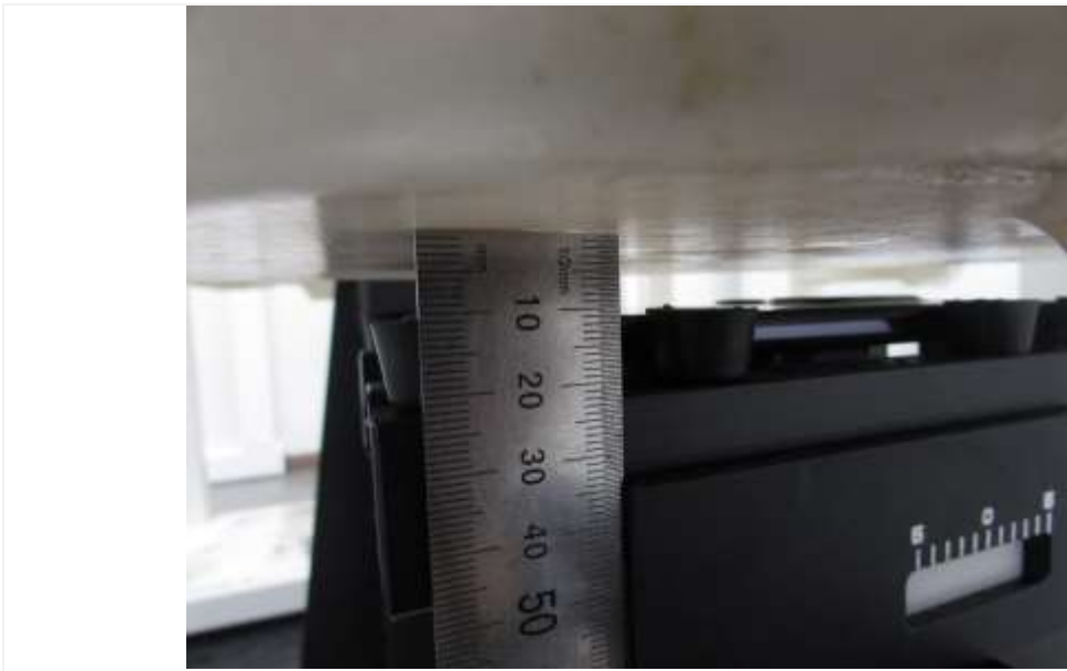
Distance of 11 mm from the EUT
