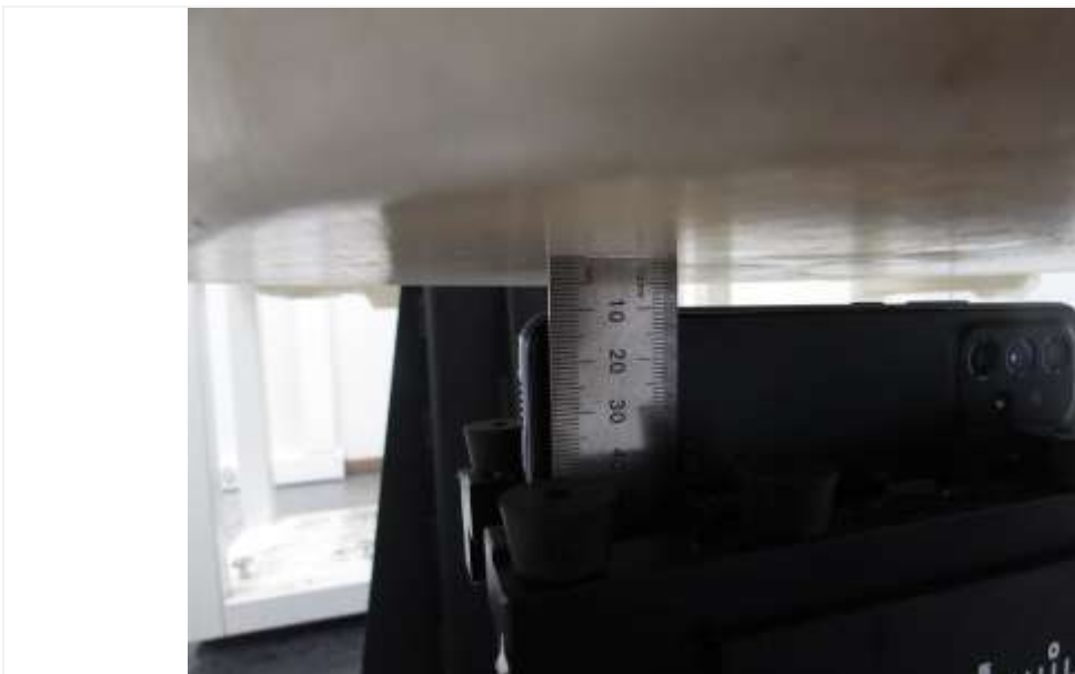
Distance of 10 mm from the EUT
