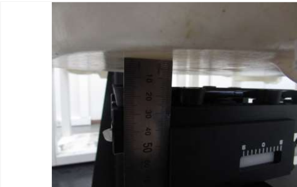
Distance of 15 mm from the EUT
