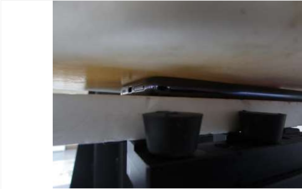
Distance of 0 mm from the EUT
