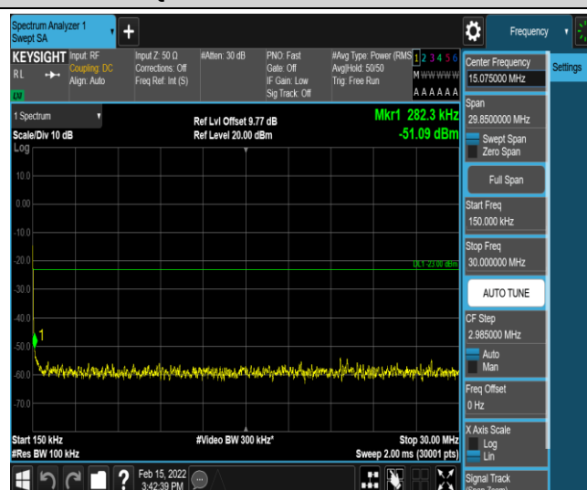
Band25-3MHz-16QAM-26055-1-0-Low-0.15-30--51.09-PASS
