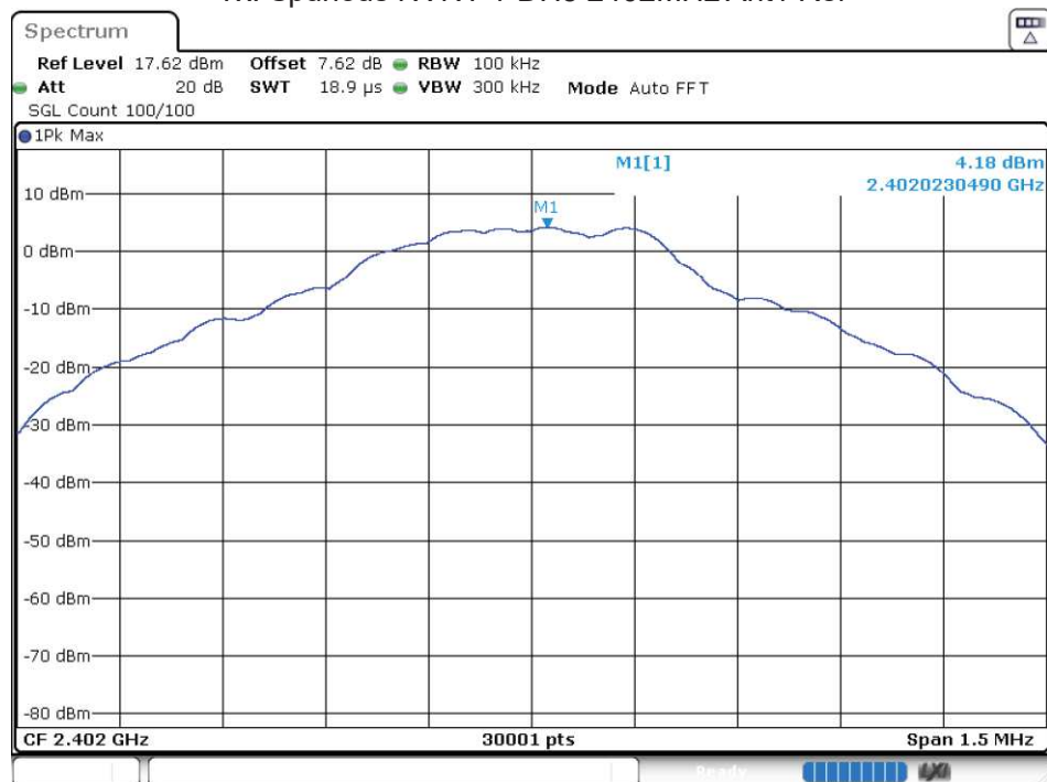
Tx. Spurious NVNT 1-DH5 2402MHz Ant1 Ref
