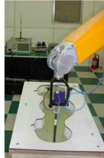
Figure 3. Photograph of the probe and the Phantom
