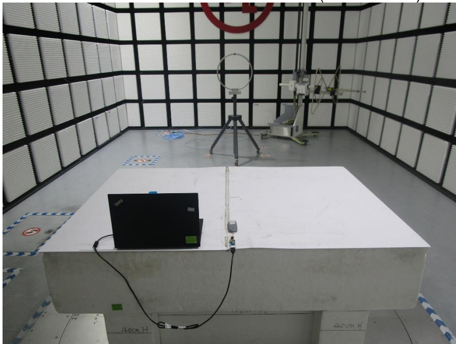
RADIATED RF MEASUREMENT SETUP (Below 30MHz)
