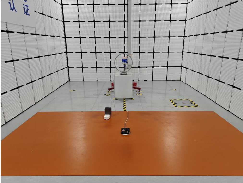
Radiated Emission Above 30MHz
