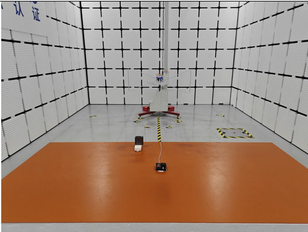
Radiated Emission Above 30MHz
