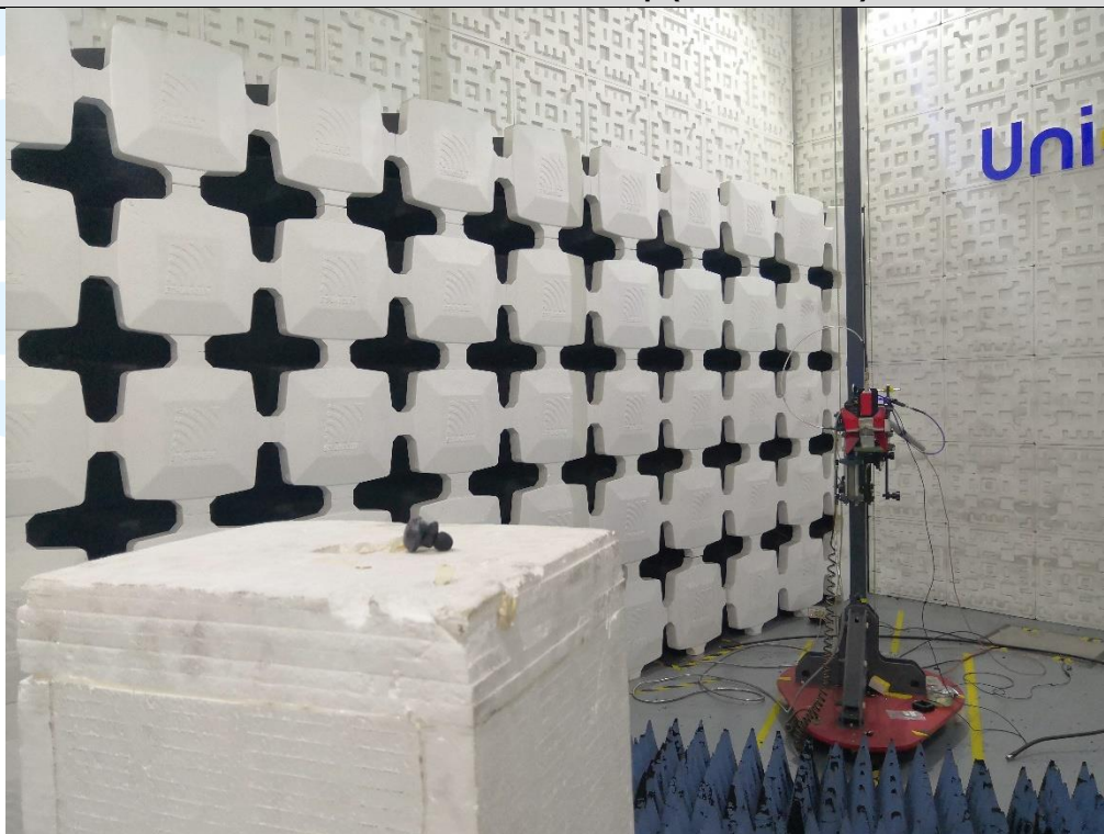
Radiated emission Test Setup (Above 1 GHz)
