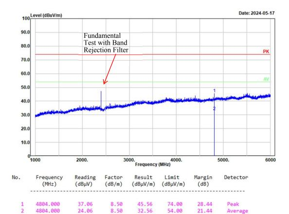
Project No.: 2403T35919E-RF Tester: Tao Zhu Polarization: vertical Note: BLE Low Channel 2402MHz
