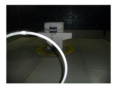
Photograph No.3 Spurious emissions measurement setup in the semi anechoic chamber in 30 -1000 MHz
