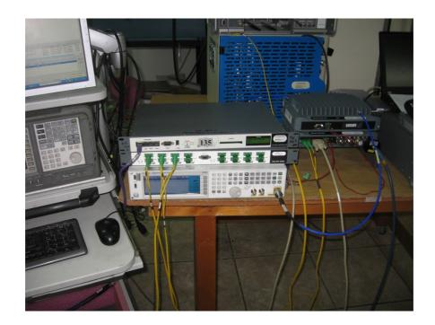
Photograph No.2 Spurious emissions measurement setup in the semi anechoic chamber below 30 MHz
