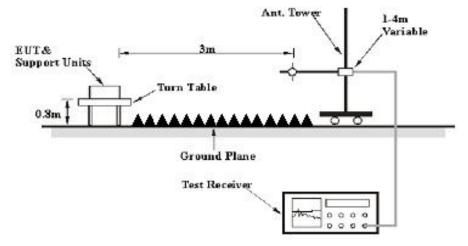
The radiated emission were performed in the 3 meters chamber test site, using the setup accordance with the ANSI C63.4-2014. The specification used was with the FCC Part 15 B Class B limits.
