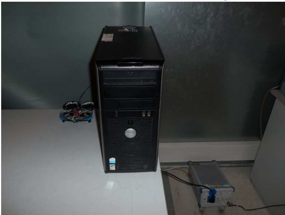
Measurement of Conducted Emission Test Set Up
