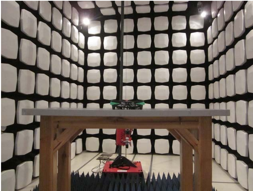
Measurement of Radiated Emission Test Set Up
