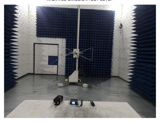
RADIATED EMISSION ABOVE 1G TEST SETUP
