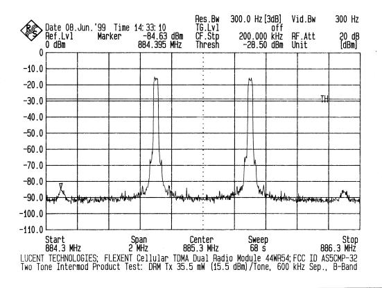
Two tones with 600 kHz separation: Channel 500, 885.00 MHz and Channel 520, 885.60 MHz Cellular TDMA Dual Radio Module output power: +15.5 dBm (36 mW) per carrier.
