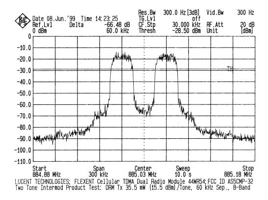
Two tones with 60 kHz separation: Channel 500, 885.00 MHz and Channel 502, 885.06 MHz Cellular TDMA Dual Radio Module output power: +15.5 dBm (36 mW) per carrier.
