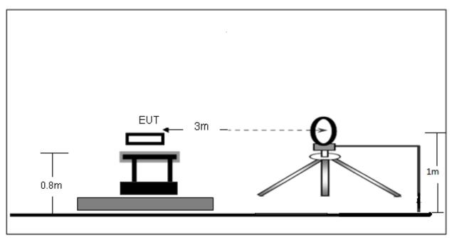
(B) Radiated Emission Test-Up Frequency 30MHz~1GHz
