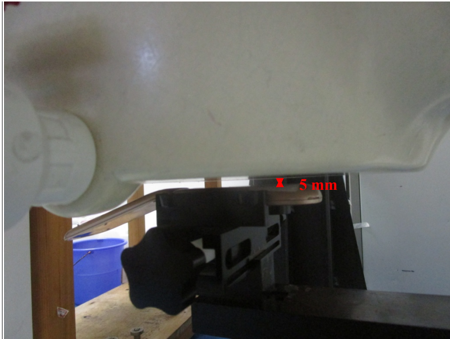
Body Worn Back Setup Photo (5mm)
