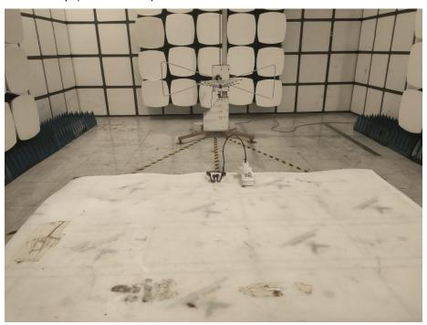
Spurious Emission Test Setup (Above 1GHz)
