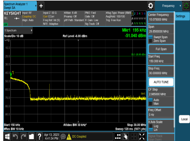
Plot 8-424. Conducted Spurious Emission Plot 150 kHz to 30 MHz
