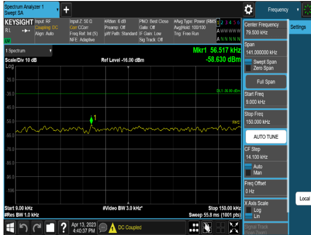
Plot 8-423. Conducted Spurious Emission Plot 9 kHz to 150 kHz
