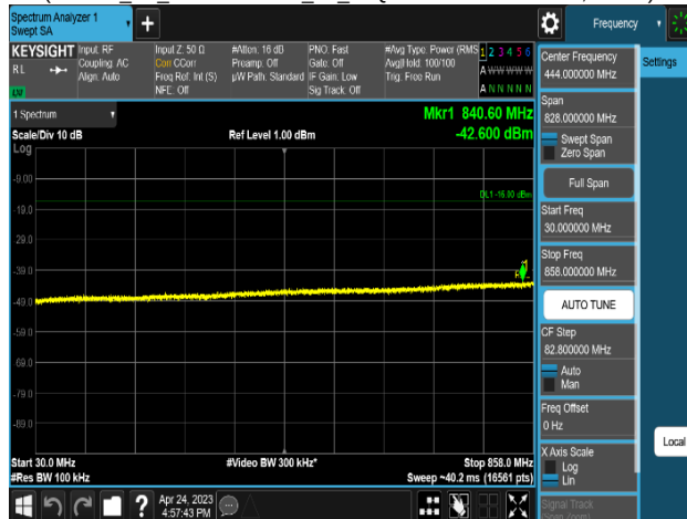
Plot 8-443. Conducted Spurious Emission Plot 30 MHz to 858 MHz
