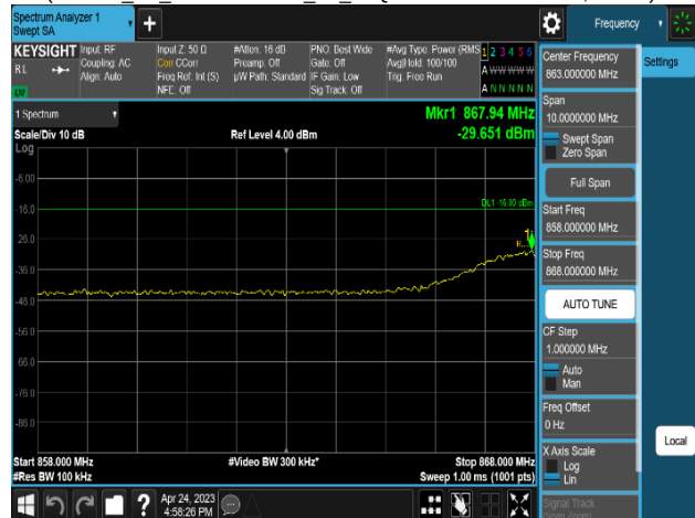
Plot 8-444. Conducted Spurious Emission Plot 858 MHz to 868 MHz
