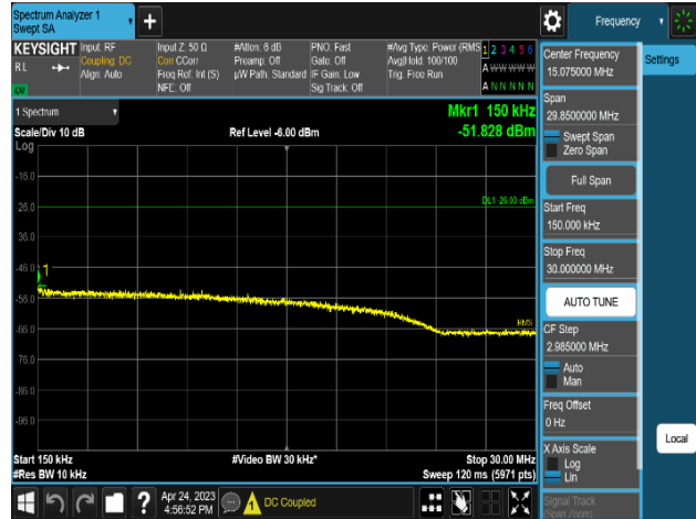
Plot 8-442. Conducted Spurious Emission Plot 150 kHz to 30 MHz
