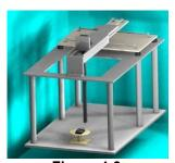
**Figure 4-3** RF Near-Field Scanner
