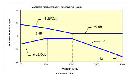
Figure 3-2 Magnetic Field frequency response for wireless devices with an axial field that exceeds -15 dB(A/m) at 1 kHz
