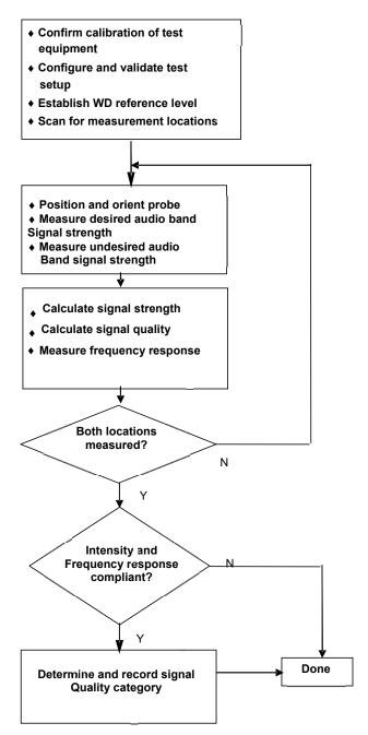
Figure 4-14 C63.19 T-Coil Signal Test Process
