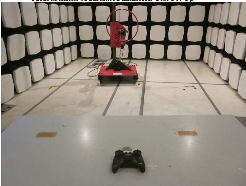
Measurement of Radiated Emission Test Set Up
