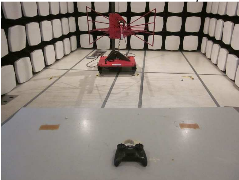
Measurement of Radiated Emission Test Set Up
