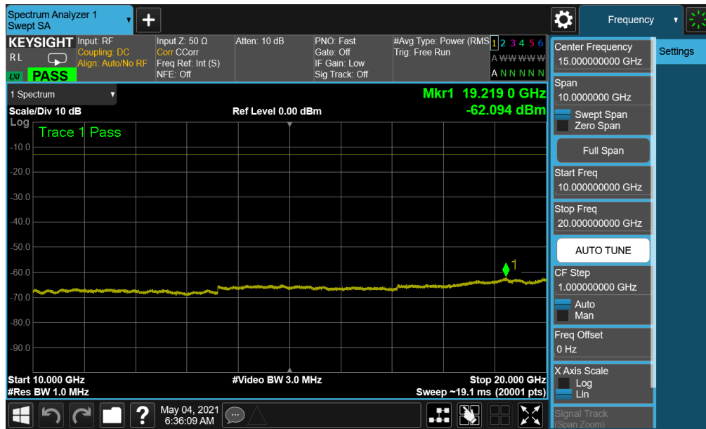
Plot 7-165. Conducted Spurious Plot (NR Band n66 - 40.0MHz - 1 RB - High Channel)
