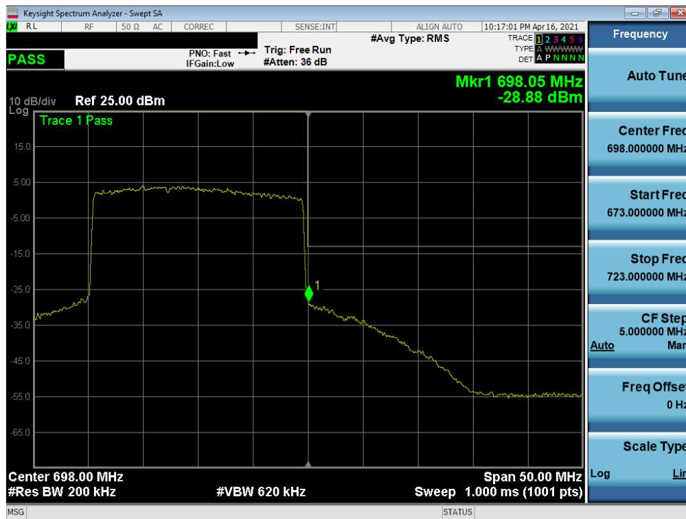
Plot 7-191. Upper Band Edge Plot (NR Band n71 – 20.0MHz - Full RB)
