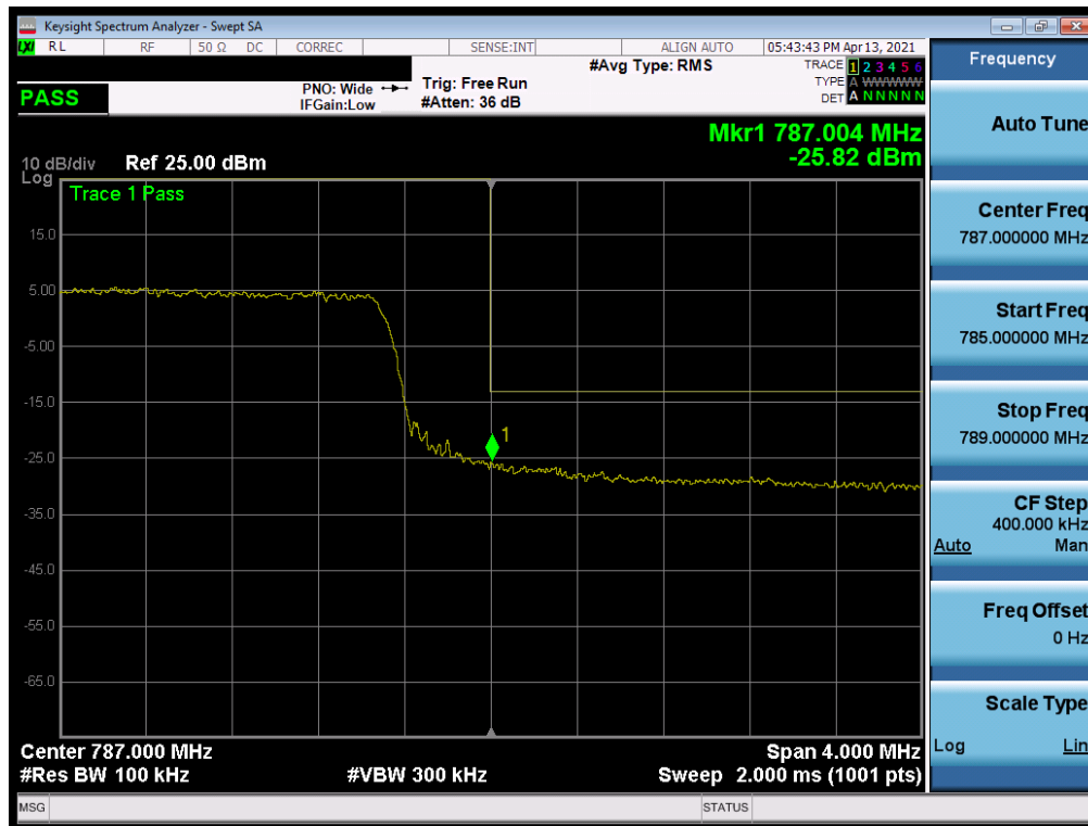
Plot 7-184. Upper Band Edge Plot (LTE Band 13 - 10MHz QPSK – Full RB)
