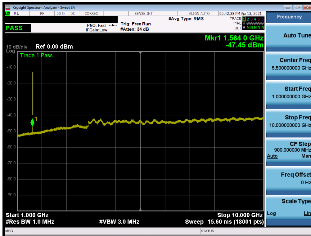
Plot 7-111. Conducted Spurious Plot (LTE Band 13 - 10MHz QPSK - RB Size 1, RB Offset 0)
