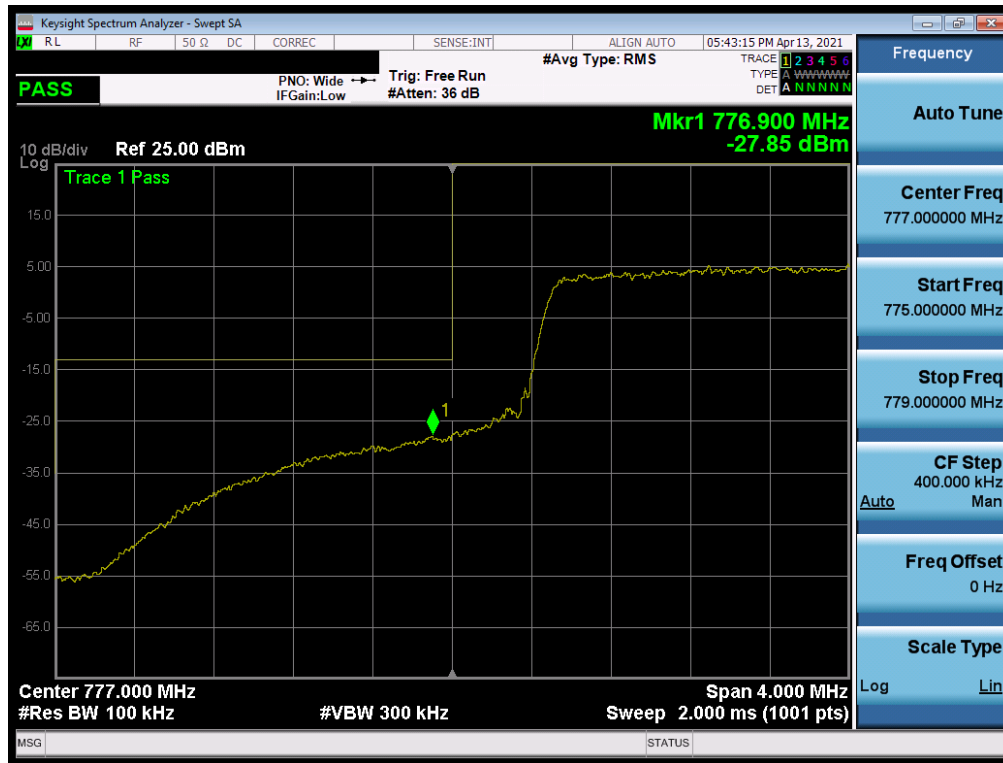
Plot 7-182. Lower Band Edge Plot (LTE Band 13 - 10MHz QPSK – Full RB)
