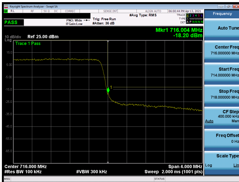
Plot 7-179. Upper Band Edge Plot (LTE Band 12 - 3MHz QPSK – Full RB)
