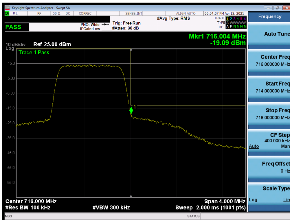
Plot 7-181. Upper Band Edge Plot (LTE Band 12 – 1.4MHz QPSK – Full RB)
