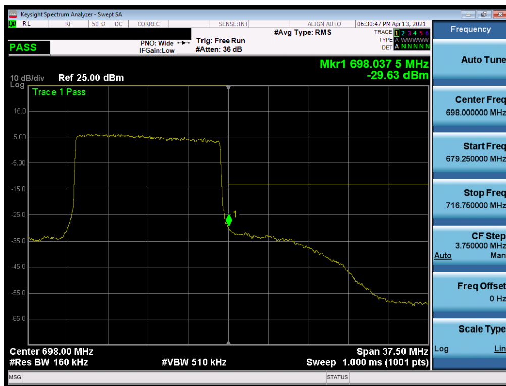
Plot 7-169. Upper Band Edge Plot (LTE Band 71 - 15MHz QPSK – Full RB)
