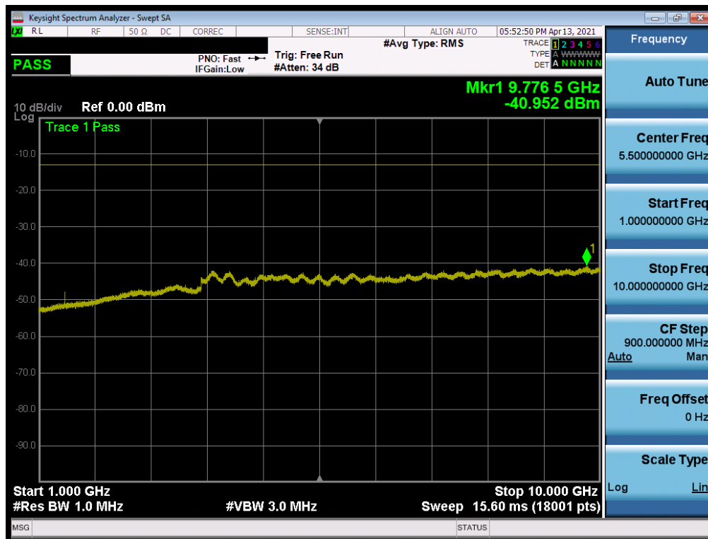
Plot 7-105. Conducted Spurious Plot (LTE Band 12 - 10MHz QPSK - RB Size 1, RB Offset 0 - Mid Channel)
