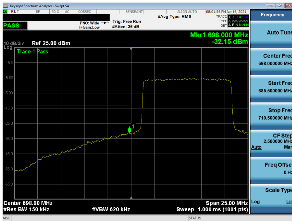
Plot 7-200. Lower Band Edge Plot (NR Band n12 - 10.0MHz - Full RB)
