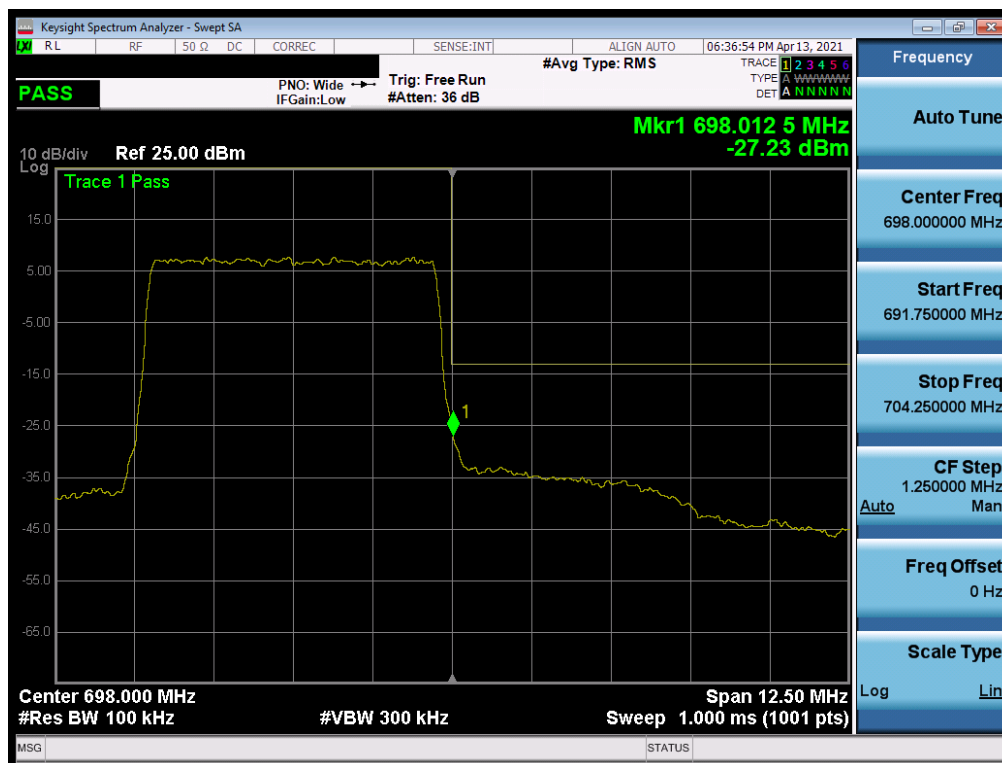
Plot 7-173. Upper Band Edge Plot (LTE Band 71 - 5MHz QPSK - Full RB)
