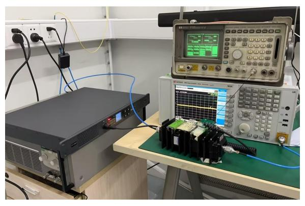
RADIATED EMISSION TEST SETUP BELOW 1GHz BY DC POWER
