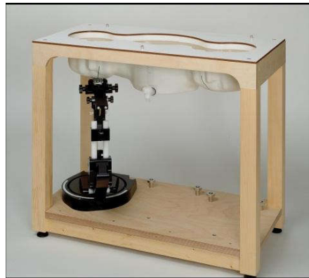
Picture C.11: SAM Twin Phantom
