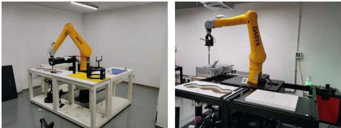
Picture D.6 Specific Absorption Rate Test Layout
