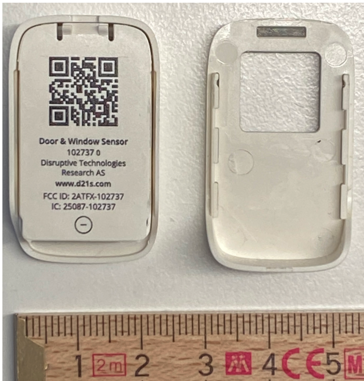
Figure 2: Picture of the back side of 102737 - Door and Window Sensor US with the mounting bracket removed.
