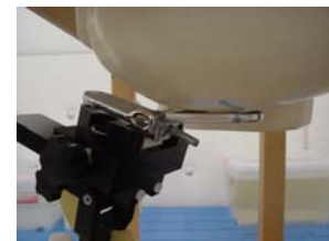
Fig. 15. Head SAR Test Setup
