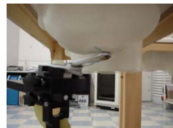
Fig. 19. Head SAR Test Setup
