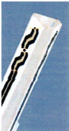
Figure 5. ET3DV6 E-field Probe
