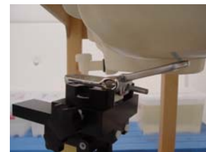
Fig. 17. Head SAR Test Setup
