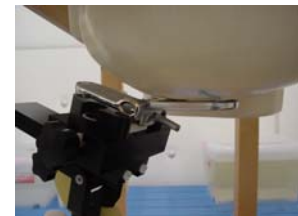
Fig. 15. Head SAR Test Setup
