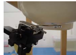
Fig. 16. Head SAR Test Setup
