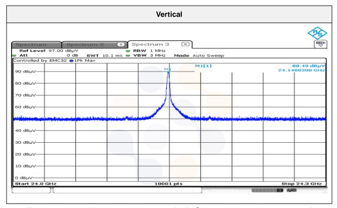
Note : The Average limit of fundamental is 107.96  $dB\mu V/m@3$  m, and the maximum measure Peak level of fundamental is 93.76  $dB\mu V/m@3$  m which is below 107.96  $dB\mu V/m@3$  m, worst case of fundamental is recorded in this report
