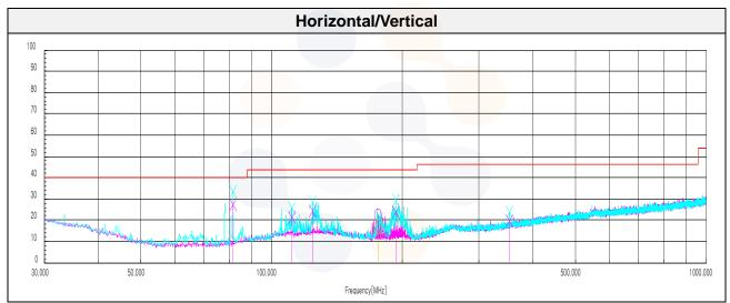
Note: The measurement results below 30  $\, \text{Mz} \,$  is greater than 20  $\, \text{dB} \,$  below the limit, so only the radiated spurious emissions from 30  $\, \text{Mz} \,$  to 100  $\, \text{GHz} \,$  were reported.
