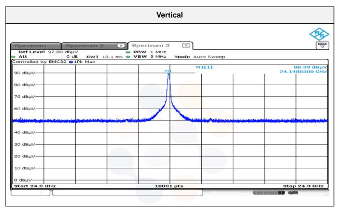
Note: The Average limit of fundamental is 107.96  $dB\mu V/m@3$  m, and the maximum measure Peak level of fundamental is 93.76  $dB\mu V/m@3$  m which is below 107.96  $dB\mu V/m@3$  m, worst case of fundamental is recorded in this report
