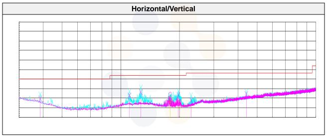
Note: The measurement results below 30  $\, \text{Mz} \,$  is greater than 20  $\, \text{dB} \,$  below the limit, so only the radiated spurious emissions from 30  $\, \text{Mz} \,$  to 100  $\, \text{Gz} \,$  were reported.
