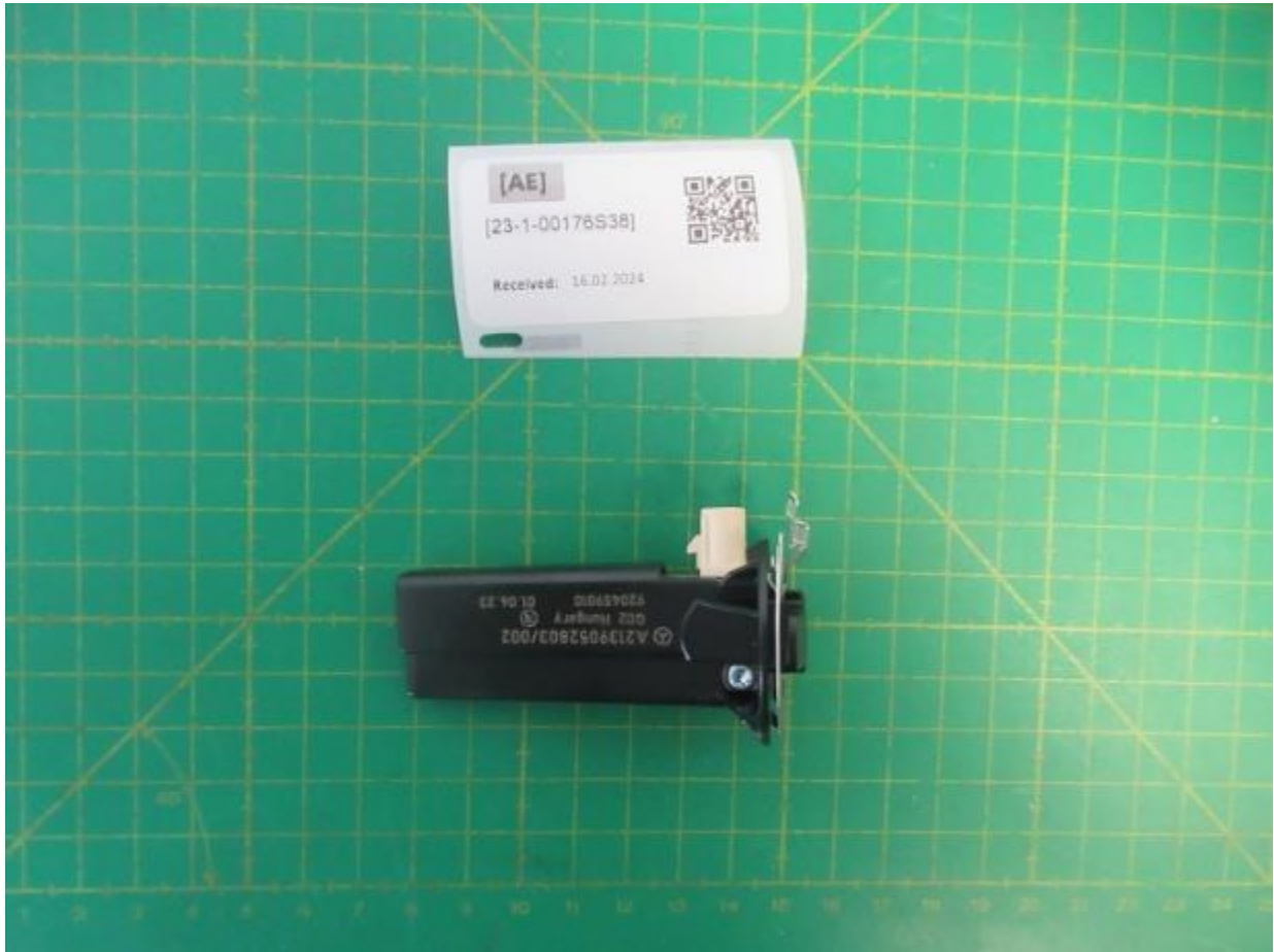
Fig. Ext.: 6 : Ext. - Front external cellular antenna
