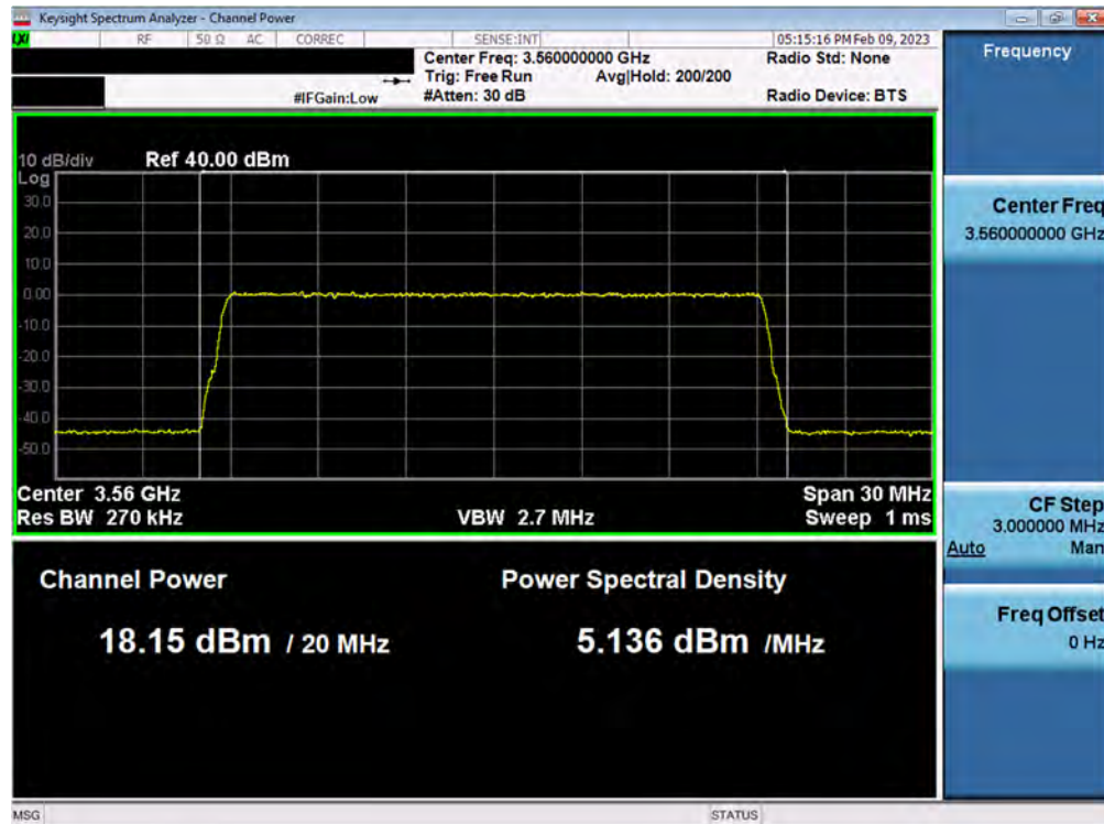
Plot 44. Conducted PSD, 3.56GHz, 20MHz BW – ANT4, SAS Granted maxEIRP 23dBm /MHz (NR)
