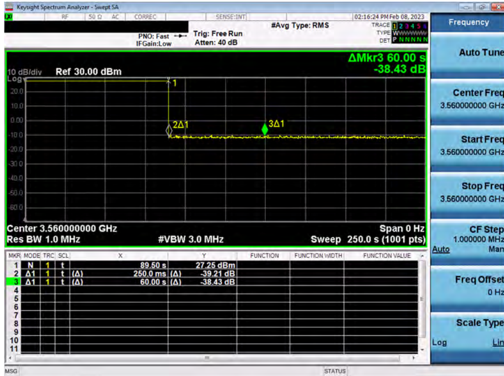
Plot 18. Conducted Measurement - RF transmission stops within transmitExpireTime + 60s. The last SAS heartbeat message is indicated by Marker 1 (X) (WINNF.FT.C.HBT.10) – NR
