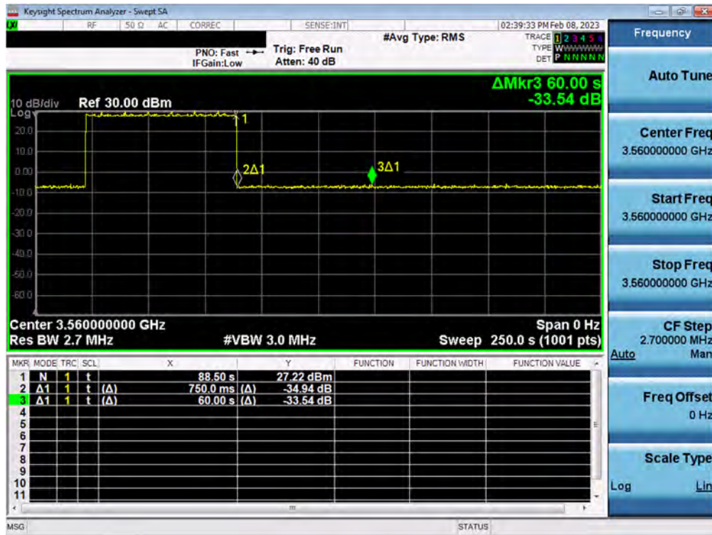
Plot 21. Conducted Measurement - RF transmission stops (WINNF.FT.C.RLQ.1) – NR
