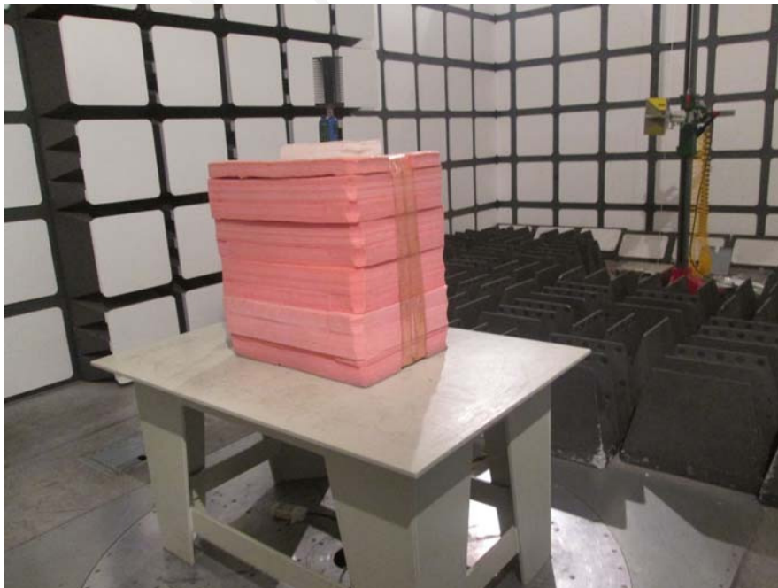
Transmitting Radiated Emissions Tested View (Above 1 GHz)
