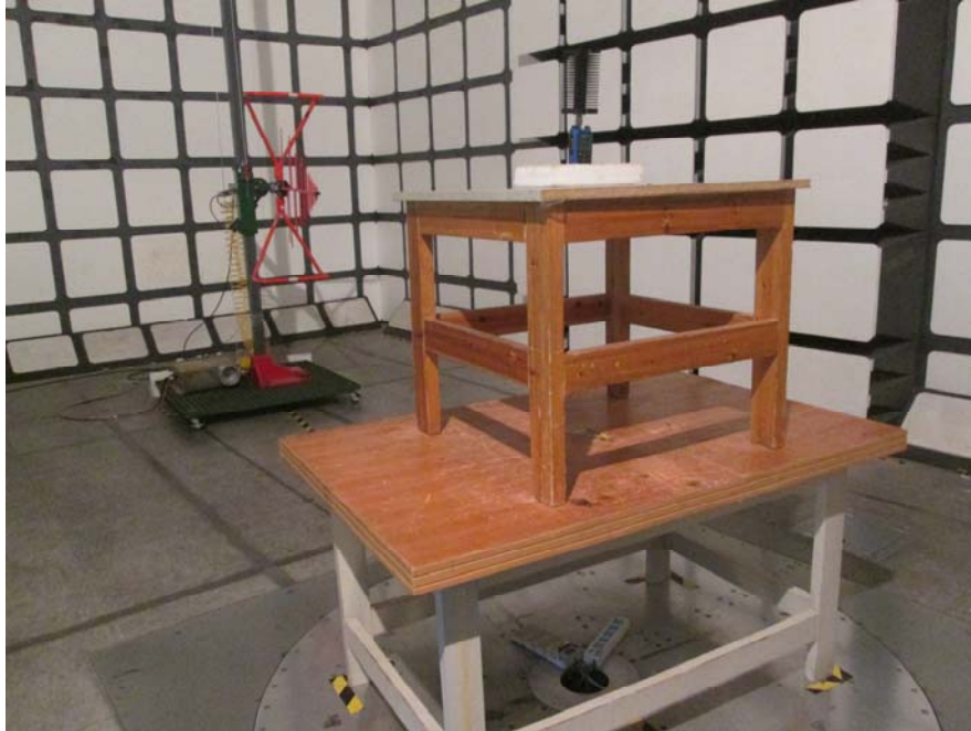
Transmitting Radiated Emissions Tested View (Below 1 GHz)
