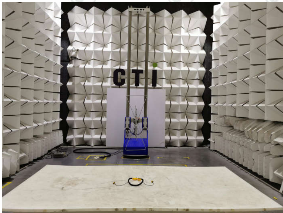
Radiated spurious emission Test Setup-1(Below 1GHz)
