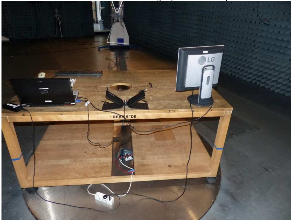
Photo 4: Test setup for radiated measurements (EUT supplied by primary AAA size 1.5 V cells, unintentional radiator §15.109, ANSI C63.4)
