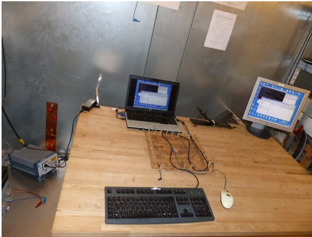
Photo 4: Test setup for radiated measurements (EUT supplied by primary AAA size 1.5 V cells, unintentional radiator §15.107, ANSI C63.4)
