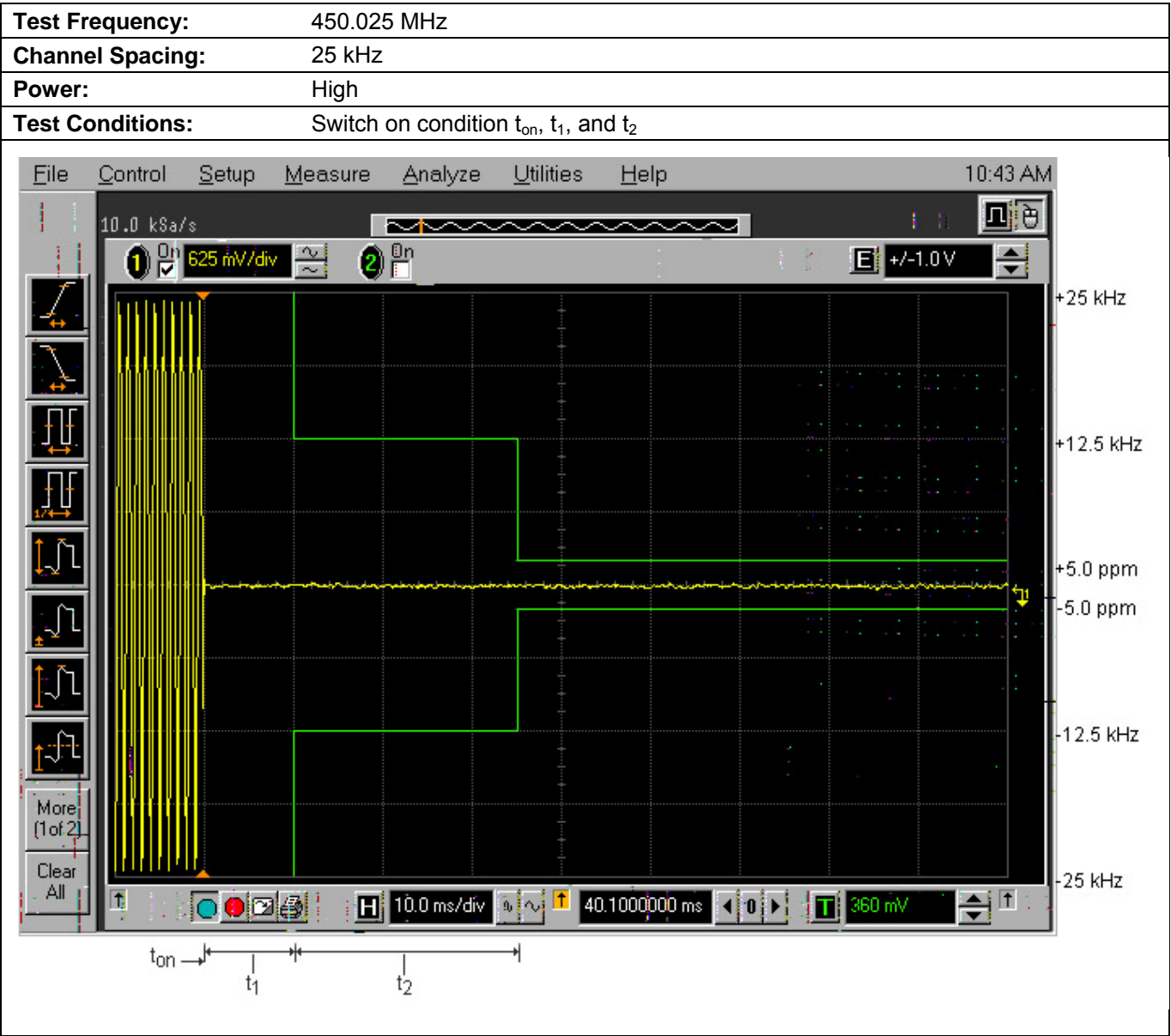
Plot 5.12.4.3. Transient Frequency Behavior for 25 kHz Channel Spacing
