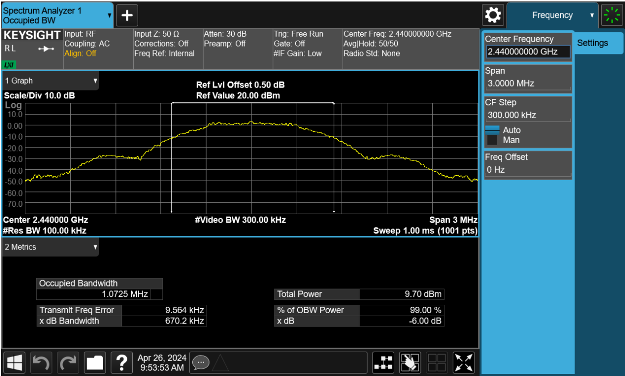
99% Bandwidth, 2440MHz, BLE-1Mbps
