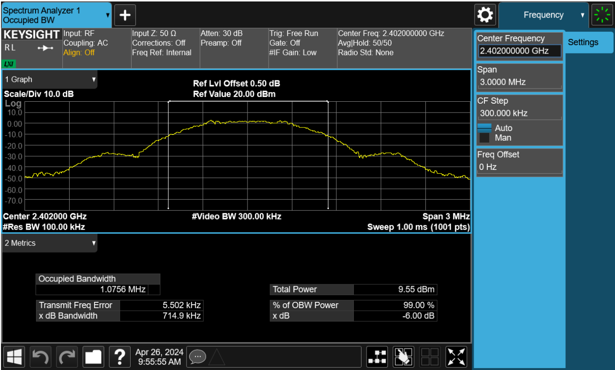
99% Bandwidth, 2402MHz, BLE-1Mbps
