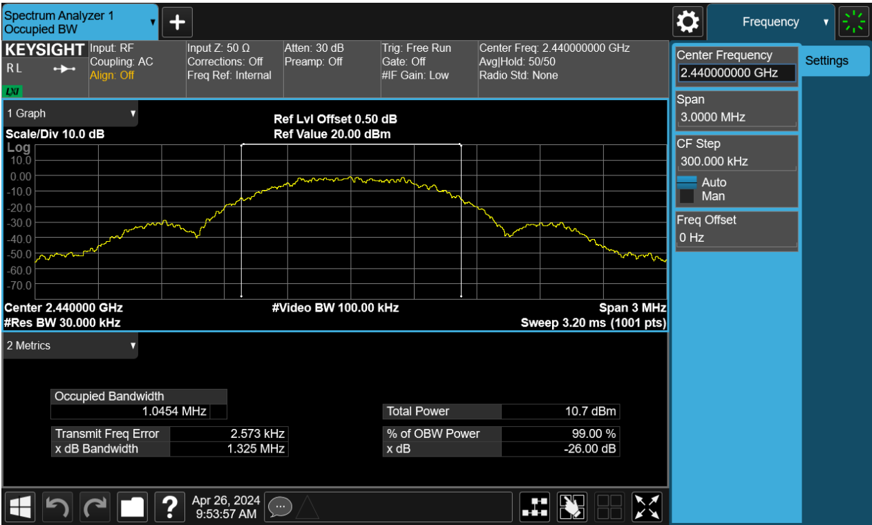
99% Bandwidth, 2440MHz, BLE-1Mbps
