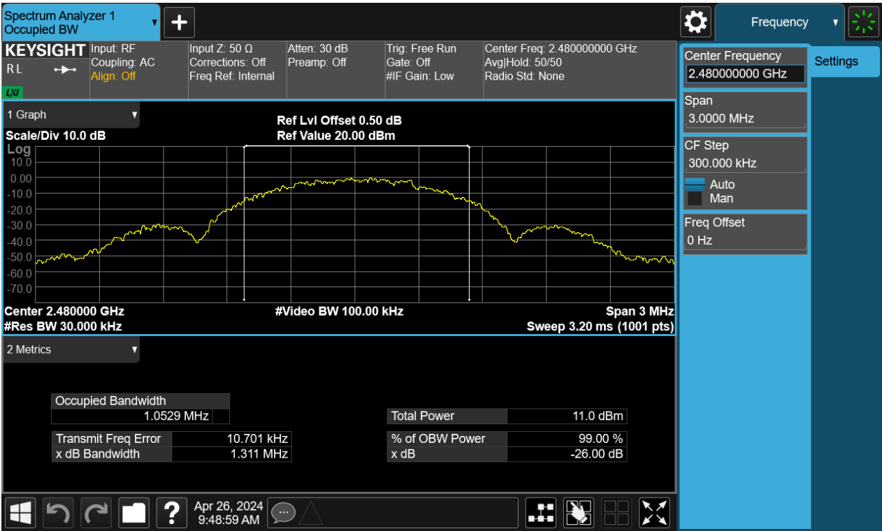
99% Bandwidth, 2480MHz, BLE-1Mbps
