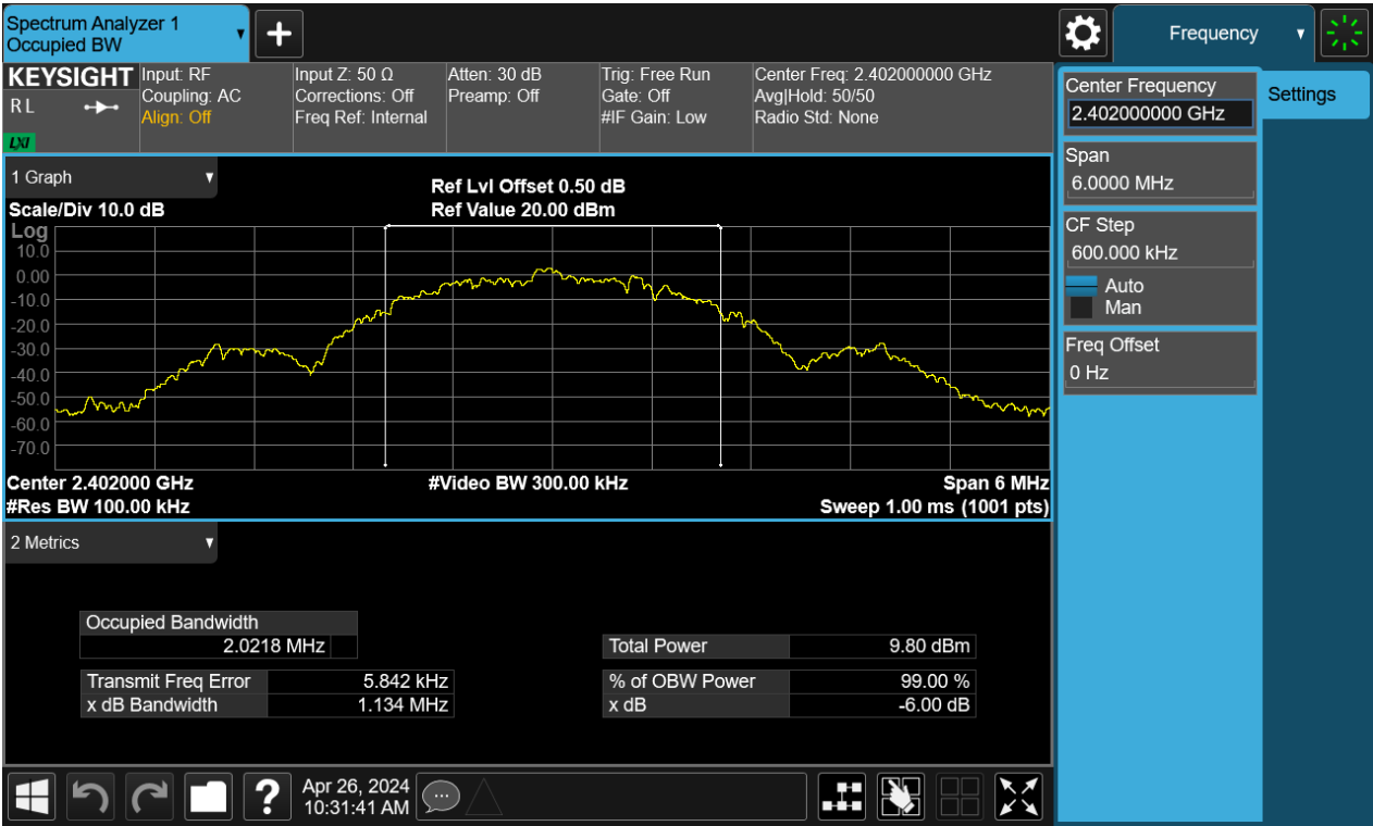
99% Bandwidth, 2402MHz, BLE-2Mbps
