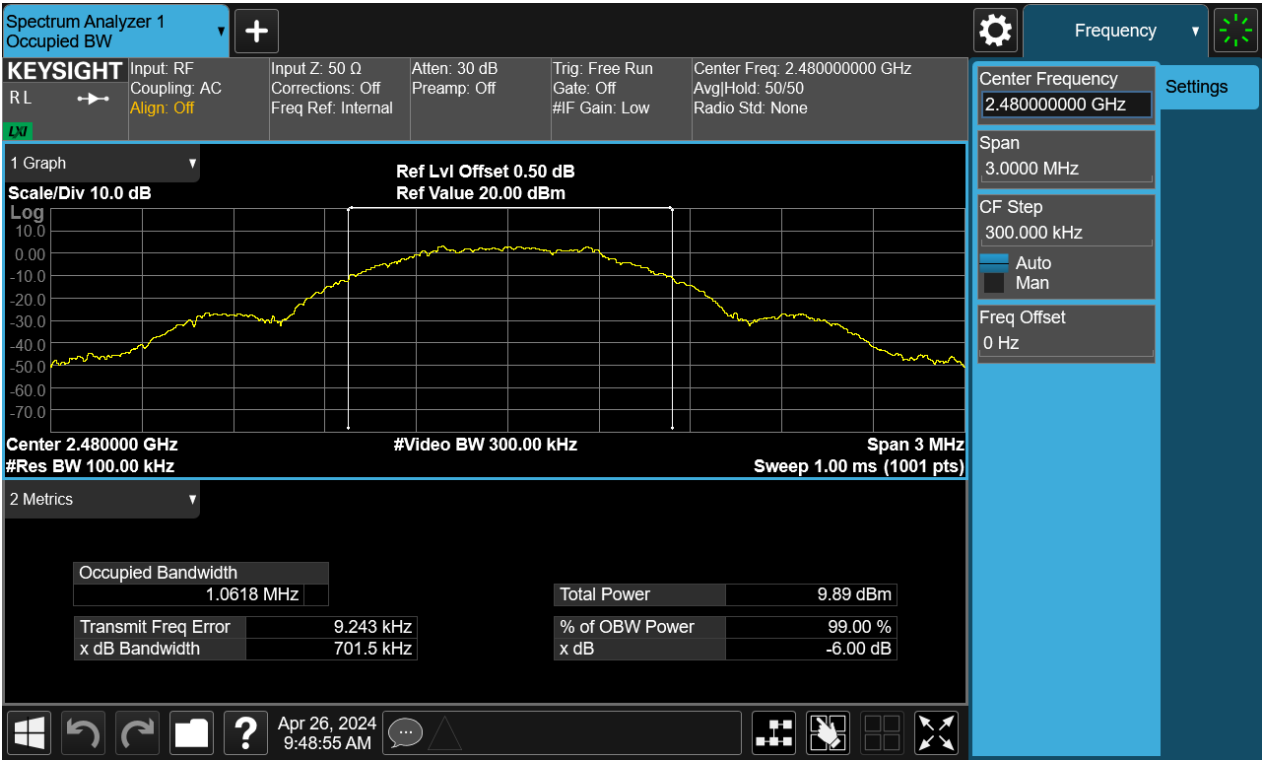
99% Bandwidth, 2480MHz, BLE-1Mbps
