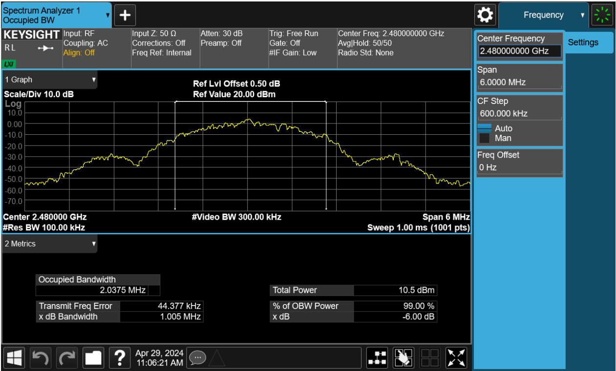
99% Bandwidth, 2480MHz, BLE-2Mbps
