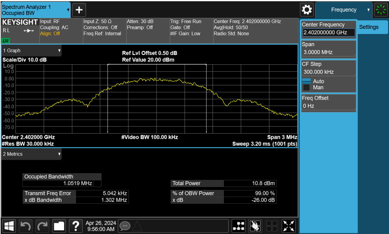
99% Bandwidth, 2402MHz, BLE-1Mbps
