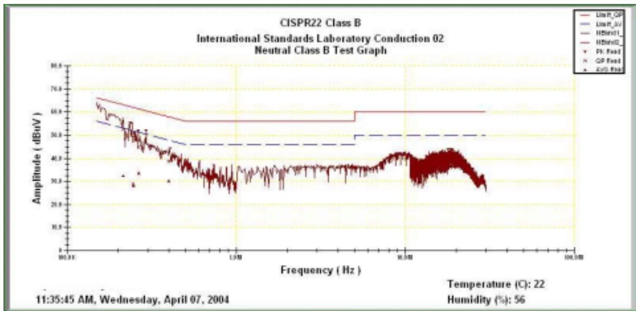
\* NOTE: During the test, the EMI receiver was set to Max. Hold then switch the EUT between Main antenna , Aux antenna Channel 9,10,12 of Normal
