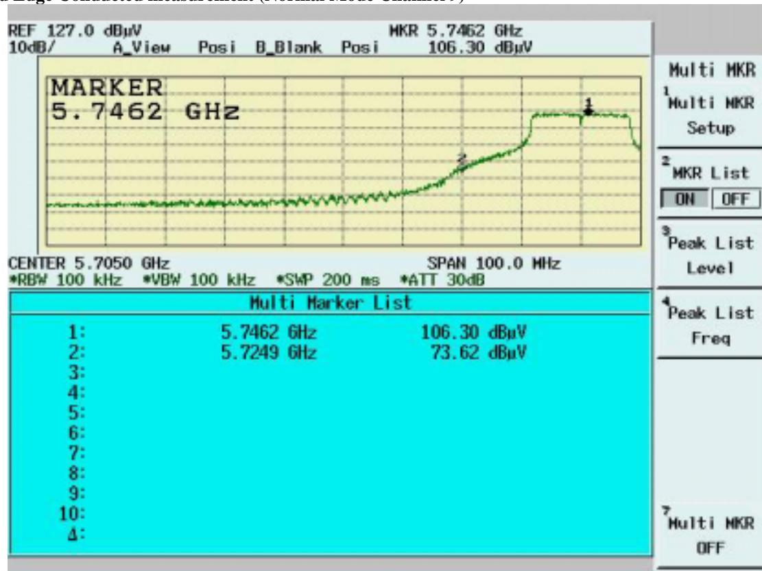
Band Edge Conducted Measurement (Normal Mode Channel 12)
