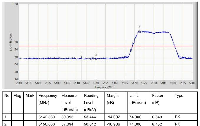
Note: Measure Level  $(dB\mu V/m)$  = Reading Level  $(dB\mu V)$  + Factor (dB)
