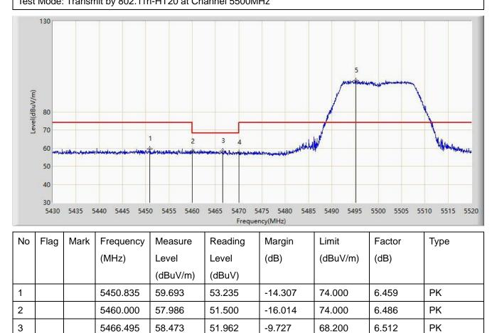
Note: Measure Level ( $dB\mu V/m$ ) = Reading Level ( $dB\mu V$ ) + Factor (dB)
