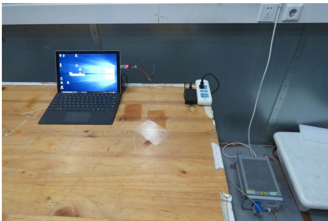
Picture 3 Conducted Emission Test Setup
