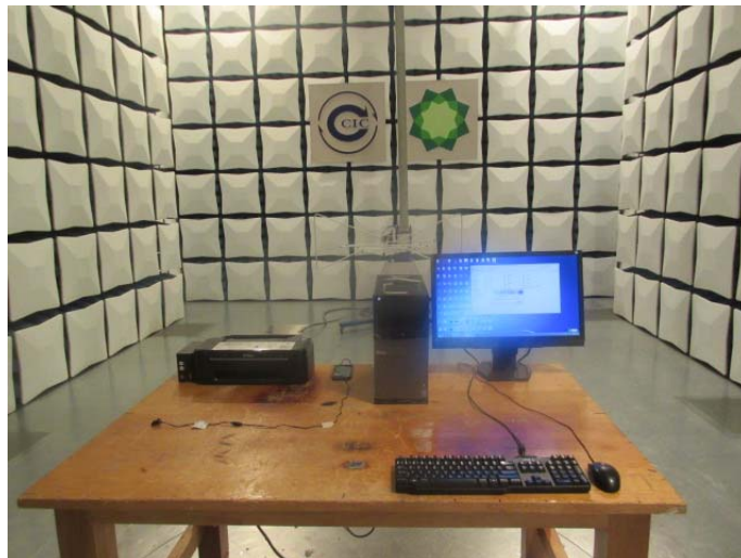
Radiated Emission (above 1GHz) Connect to PC
