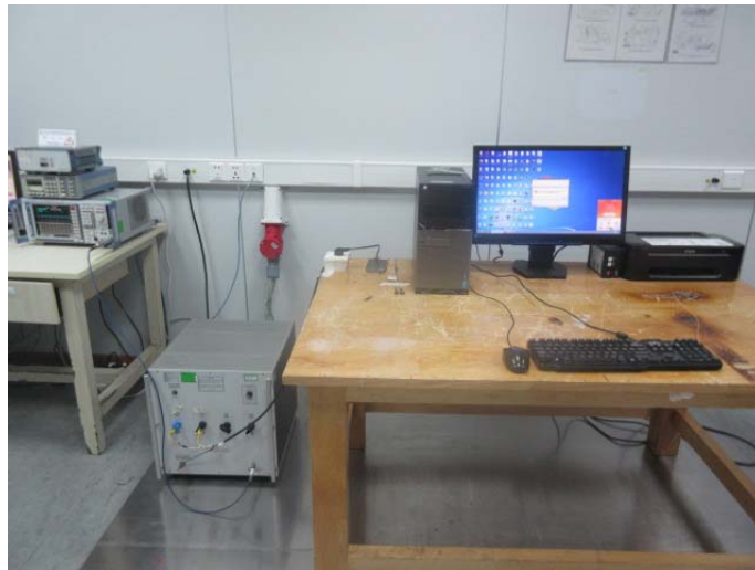
Radiated Emission (30MHz-1GHz) Connect to PC
