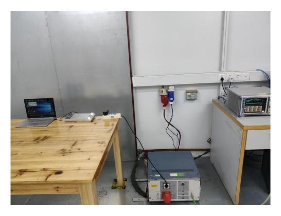
FCC RADIATED EMISSION TEST SETUP
