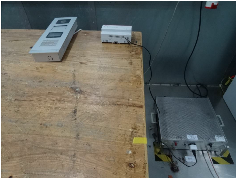
Setup photo of conducted emission (150KHz-30MHz)
